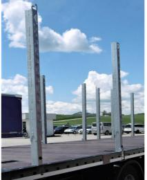
Telescopic stanchions: Check the weld seams for cracks
