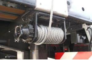
Wire tensioners: Check operability and proper mounting
