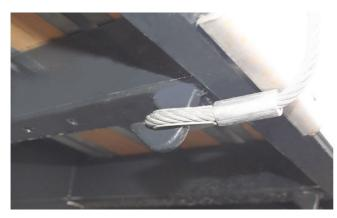
Wire tensioner holding hooks: Check the weld seams for cracks
