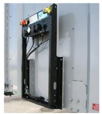
Tool holder: Check that all rivets and screws are tight
