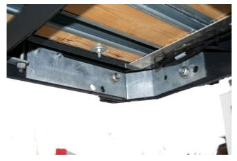
Check that the screw fitting of the inner corner post is tight
