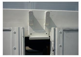
Stanchion bearings: Check the weld seams for cracks
