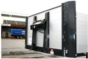
Tool holder: Check that all rivets and screws are tight
