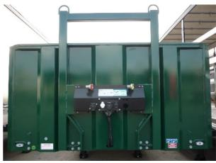
Check that the screw fittings are tight Check the weld seams for cracks
