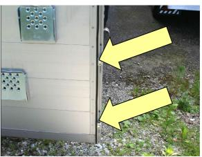
Check that the holding hooks on both sides are tight
