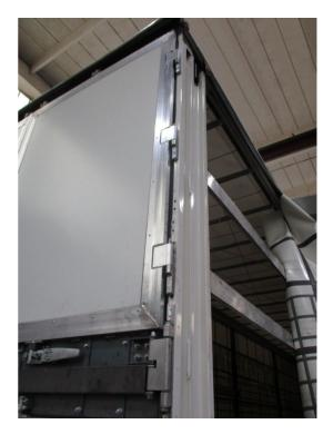
Bottom, central and top rear door: Check latches and locking pins for wear, damage and correct operability; check that the screws are tight
