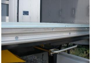
Check bottom guide rail for wear and correct operability, Check that screws fittings are tight.
