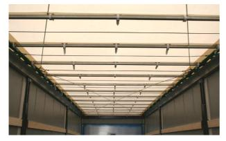
Wires and wire mounts: Check for damage and proper operability
