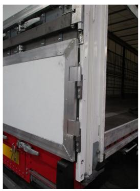
Check the hinges for operability and damage Check the hinge mounts for damage and tight fit
