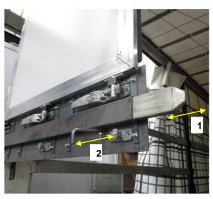
Check cross latching bolt (1) and actuation (2) for wear, damage and correct operability
