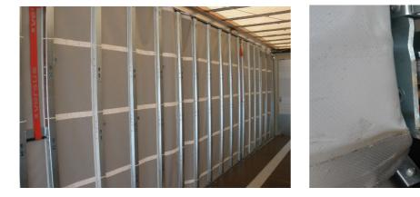
Visual inspection of Quick Slider for plastic deformation etc. Check bottom joints and carriages for wear and correct operability, check that screw fitting is tight
