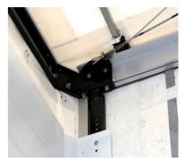
Check that all rivets and screws are tight
