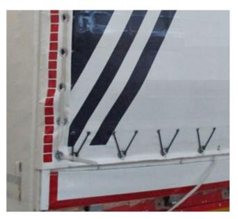
Check that strap feedthrough sleeves are not ripped, Check the rubber bands for rips.
