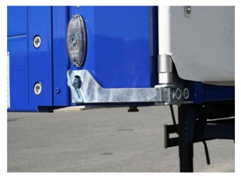
Front quick lock: Check attachment and correct operability. Check tarpaulin draw tube adapter for damage
