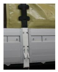
Side walls: Check that rivets are tight, check that latches are tight
