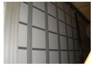
Rola-Safe sliding tarpaulin: Check steel straps for deformation
