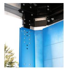
Front corner posts: Check that rivets are tight
