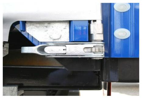
Rear tensioning gear: Check correct operability, check tarpaulin draw tube adapter for damage
