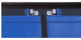
Top rear door: Check locking pin for damage and and that screws are tight
