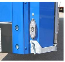
Corner post: Check that all rivets and screws are tight
