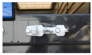
Bottom rear door: Check locking pin for damage and that screws are tight
