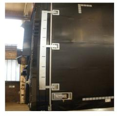
Quick Lock door: Check latch for wear and correct operability, mountability on rear corner post
