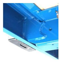
Interior stanchion bearings: Check the weld seams for cracks
