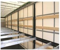
Side tarpaulin: Check the weld seams Front corner post: of strap reinforcements for cracks and damages
