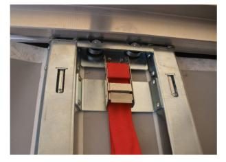
Check top and bottom carriages for wear and correct operability. Check that all rivets and screws are tight
