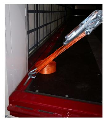
Load securing equipment: Check holding rings, tension belt and tension belts for deformation and cracks.
