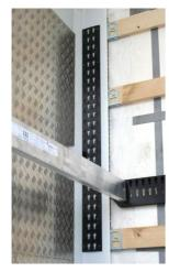
Front corner post: Check that the rail rivets are tight
