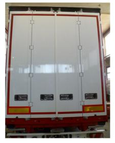
Hinges, latches etc.: Check for wear and correct operability
