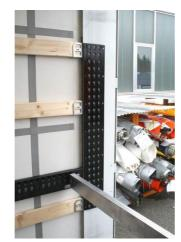
Rear corner post: Check that the rail rivets tight
