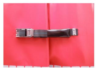
Vertical tarpaulin fold: Check tensioners for damage and correct operability
