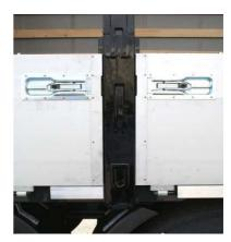
Side walls: Check that rivets are tight, check that latches are tight
