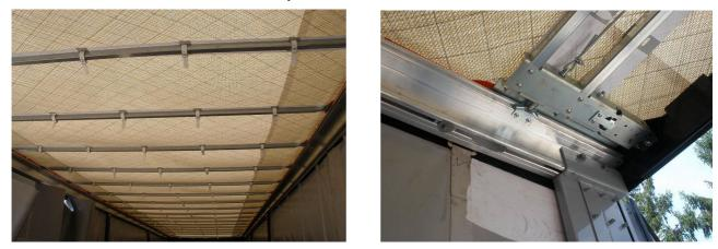
Aramid reinforced roof tarpaulin: Check for damage and correct attachment
