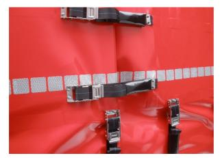
Vertical tarpaulin fold: Check tensioners for damage and correct operability
