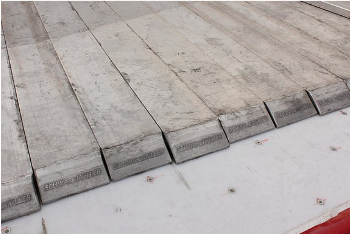
Cargo Floor sliding floor, hydraulic movement with 21 floor profiles for loading and unloading
