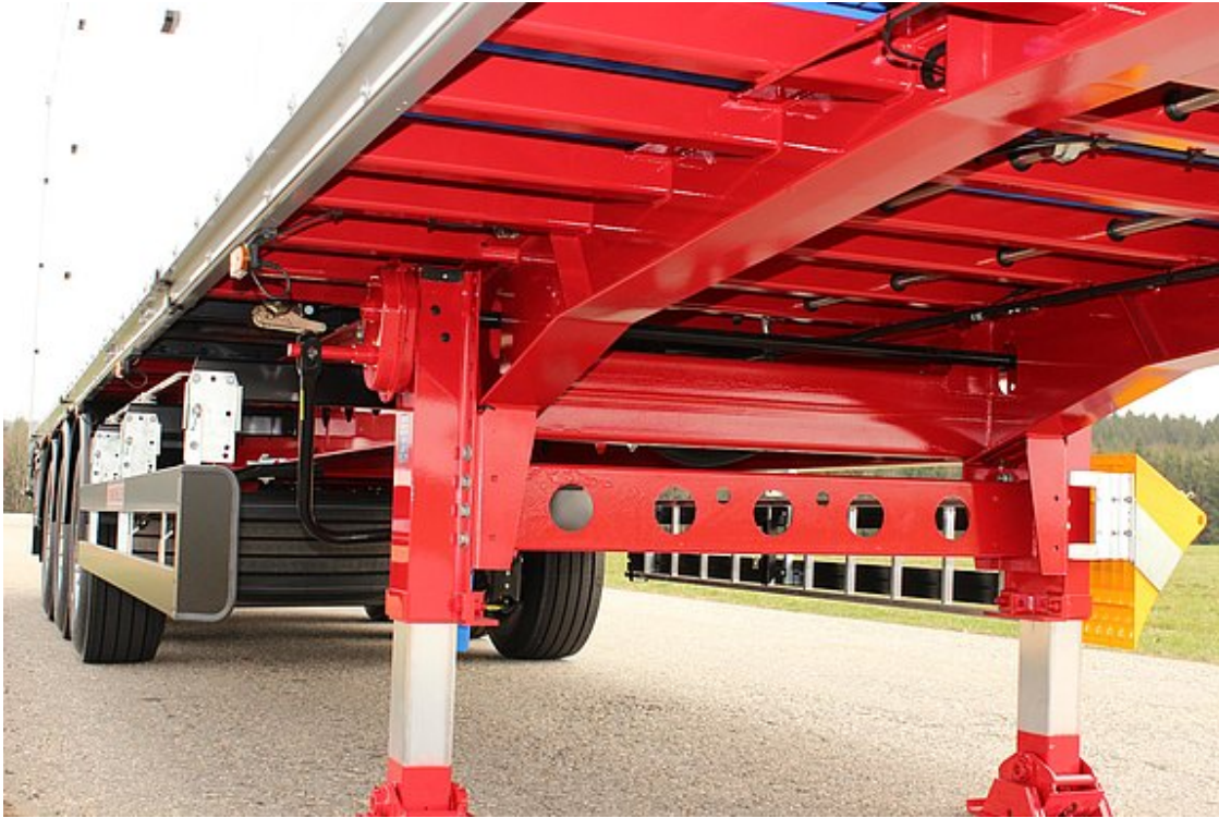
Torsionally rigid, continuous steel frame construction
