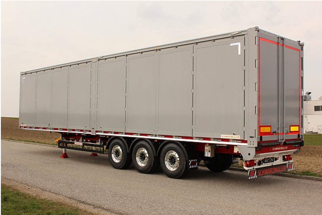
3-axle sliding floor semitrailer with side doors
