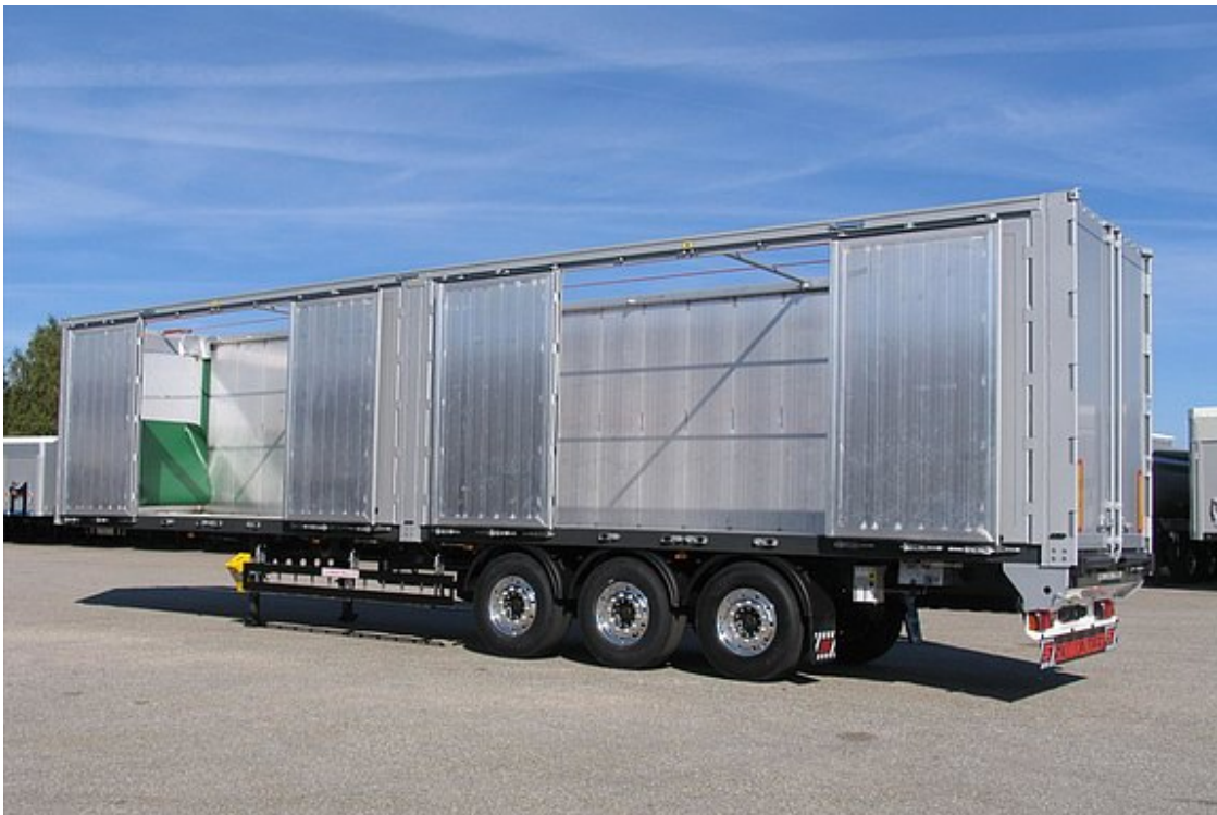
Left side with 2 4-leaf doors, for (un)loading on the side
