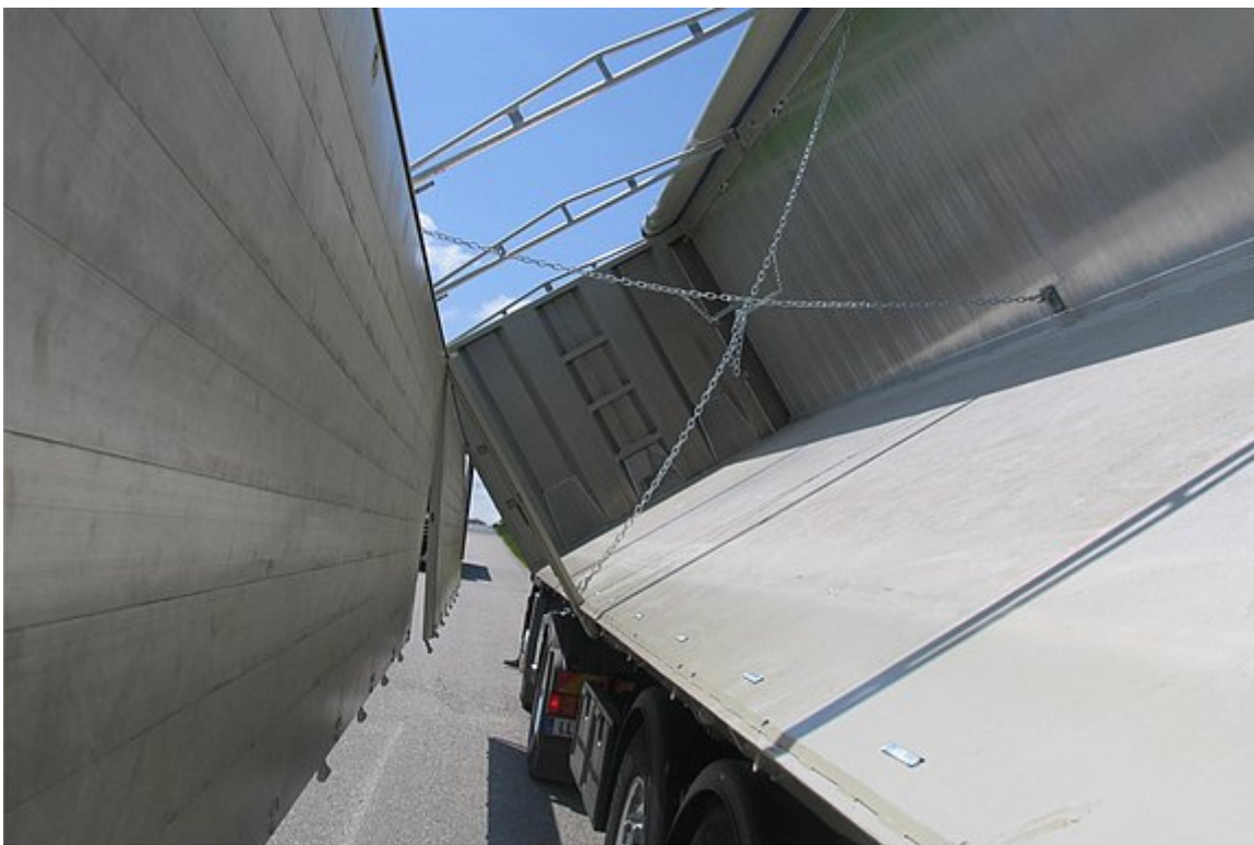
2-part side walls incl. removable centre column for maximum loading width
