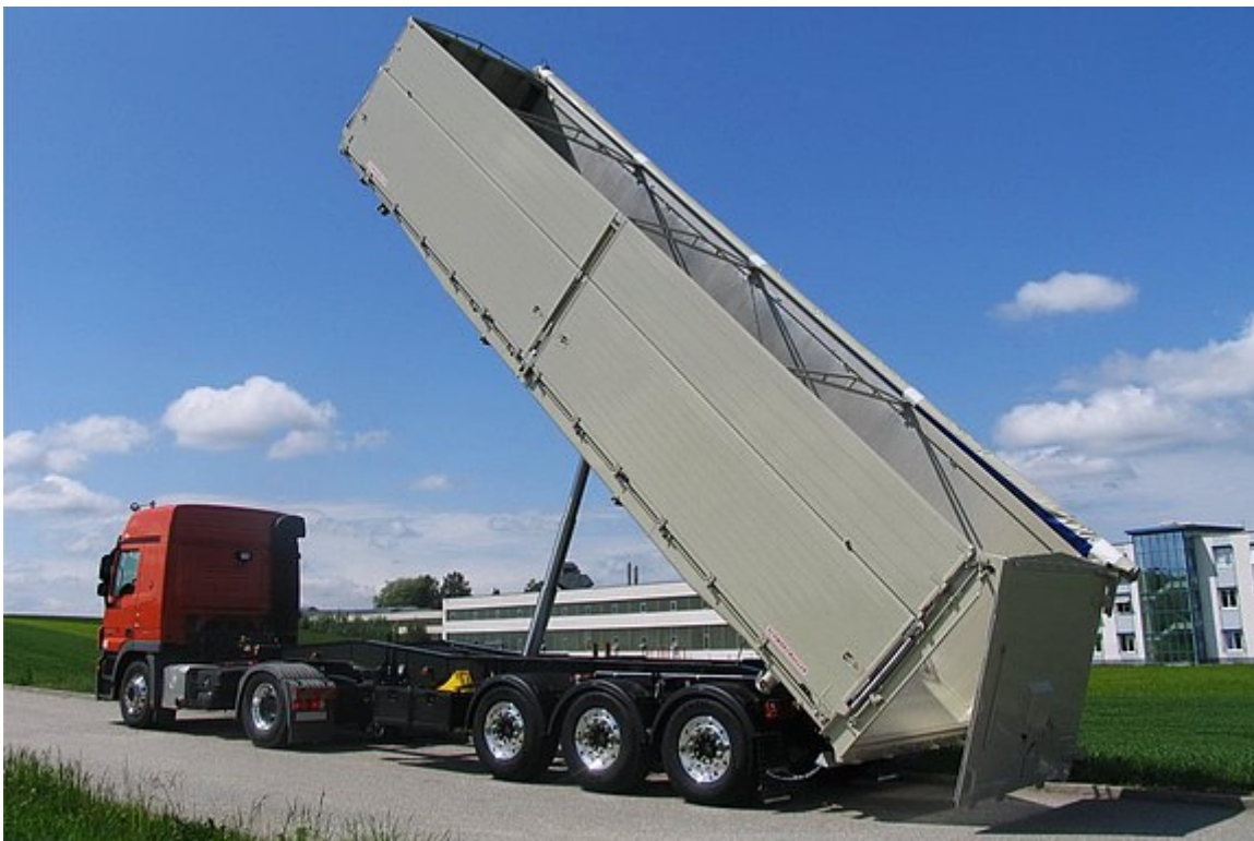
3-axle large-scale aluminium hollow profile tipper semitrailer for (un)loading and tipping to the left and rear in the direction of travel
