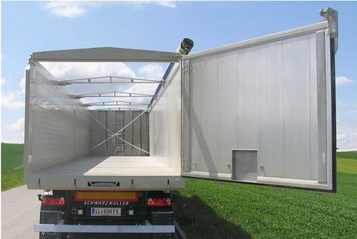
Combined rear wall - single-leaf, fully opening door and hinged with autom. pneumatic lock
