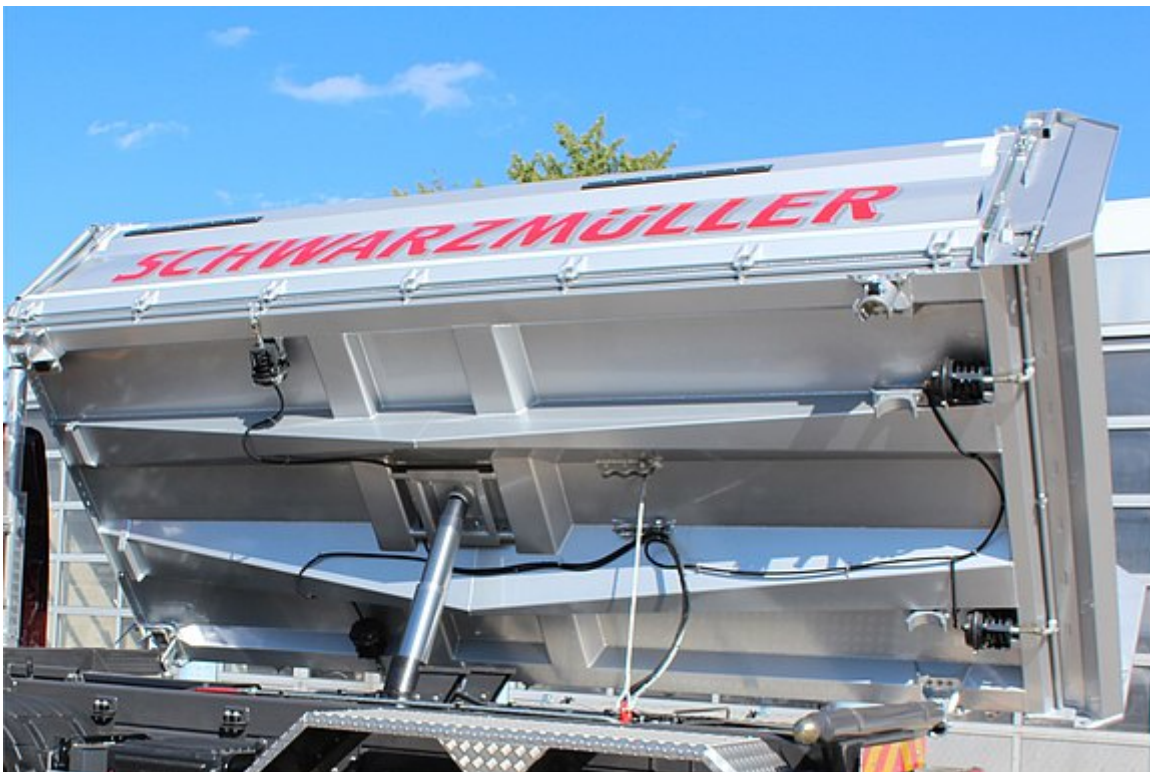
Tipper body design with conical trapezoidal profile side members in high-strength, lightweight design with small bottom panels for high dent resistance and shock absorption
