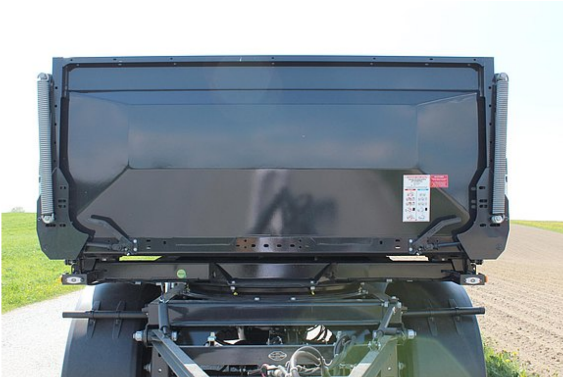
Fixed steel-sheet front wall
