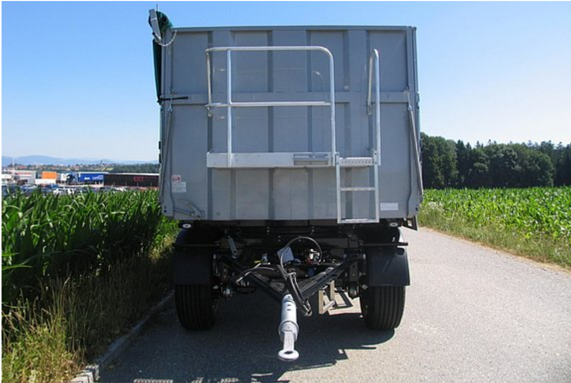
Front view - fixed steel sheet front wall and drawbar with silent bushing
