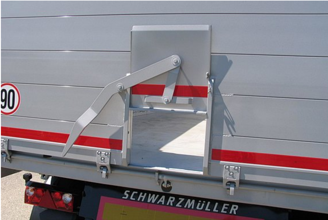
OPTIONAL: Grain feeder approx. 400/400 mm with side-mounted dosing lever in rear wall and water guard plate
