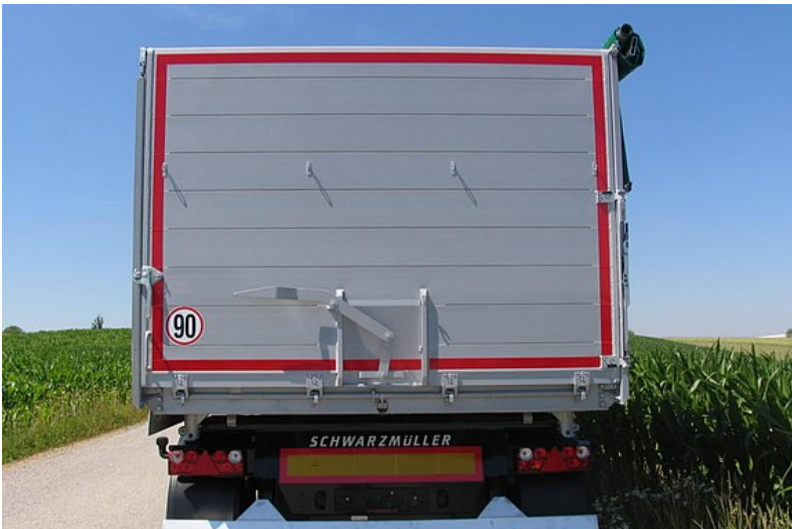
Aluminium hollow profile rear wall, folding and hinged with man. central locking and OPTIONAL pivoting as door leaf
