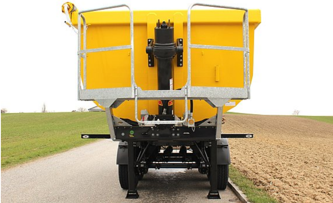
Standing platform on the front wall for operating the roller tarpaulin
