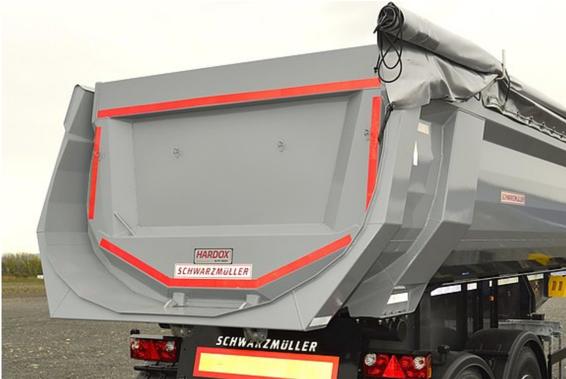
Steel rear wall = hinged wall with recessed bearing and autom. mech. dual-hook central locking
