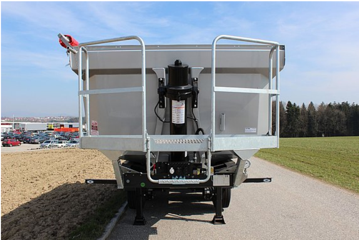
Standing platform on the front wall for operating the roller tarpaulin
