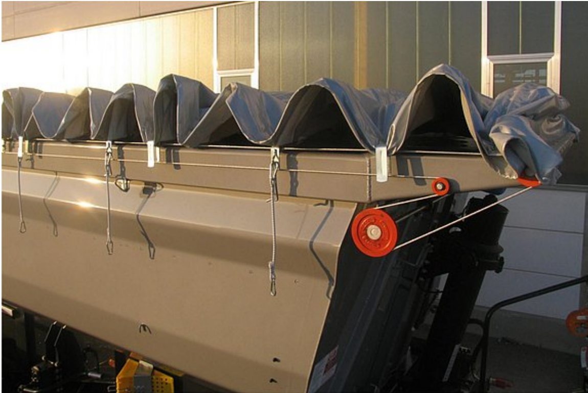
Roll-on cover - operated either manually or using an electrical remote control
