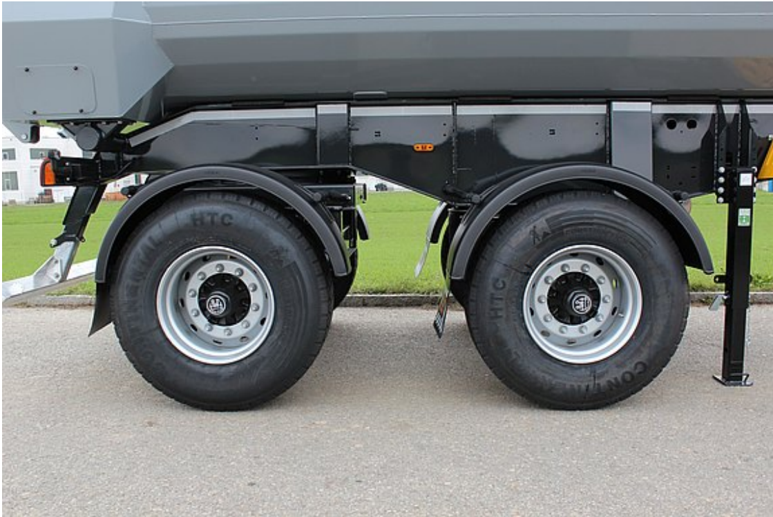
Axles with a wheelbase of 1,810 mm
