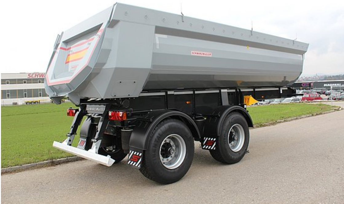
2-axle steel segment tipper semitrailer - wheelbase 1,810 mm
