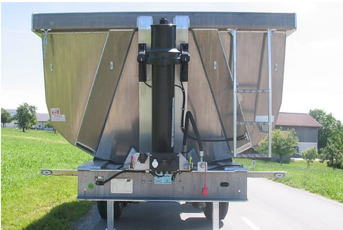
Inclined front wall with hard chrome-plated, high-grade front tilt cylinder
