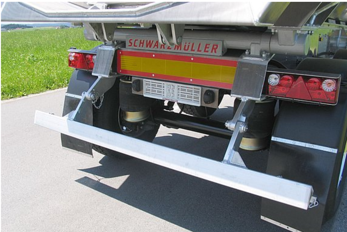
Foldable aluminium trapezoidal underride protection
