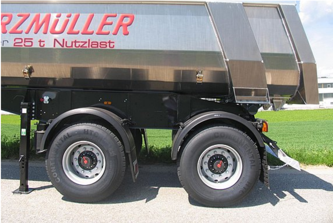
Axles with a wheelbase of 1,810 mm
