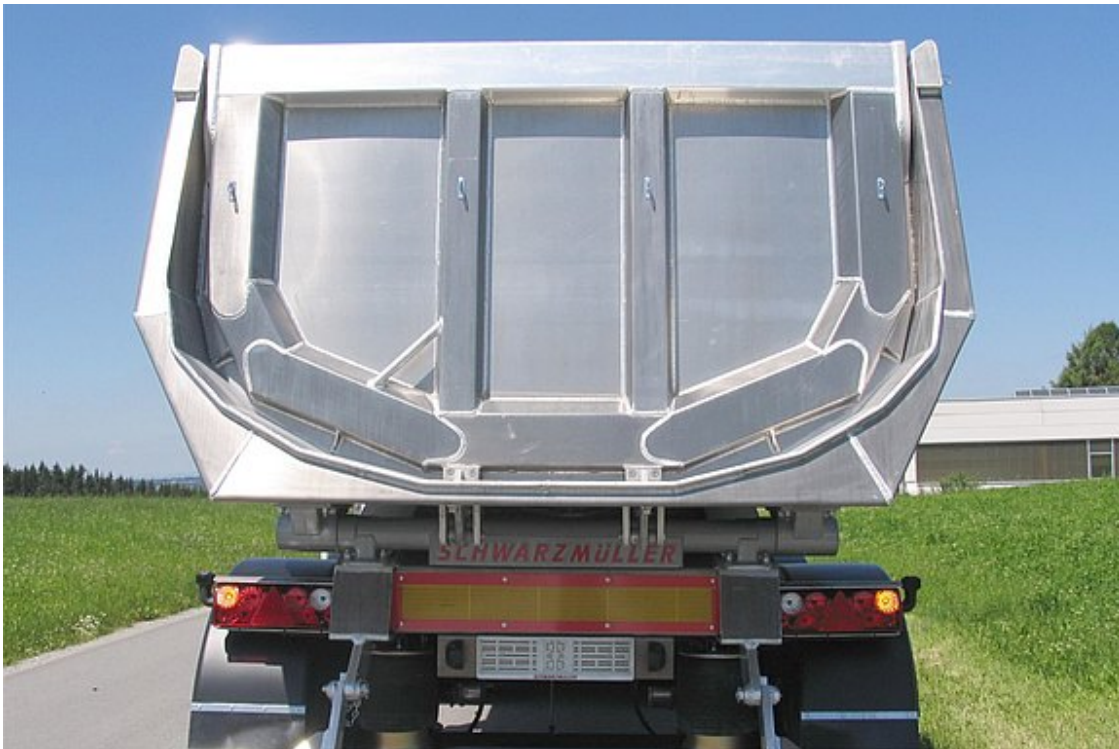
Rear wall = hinged wall with recessed bearing and autom. mech. dual-hook central locking
