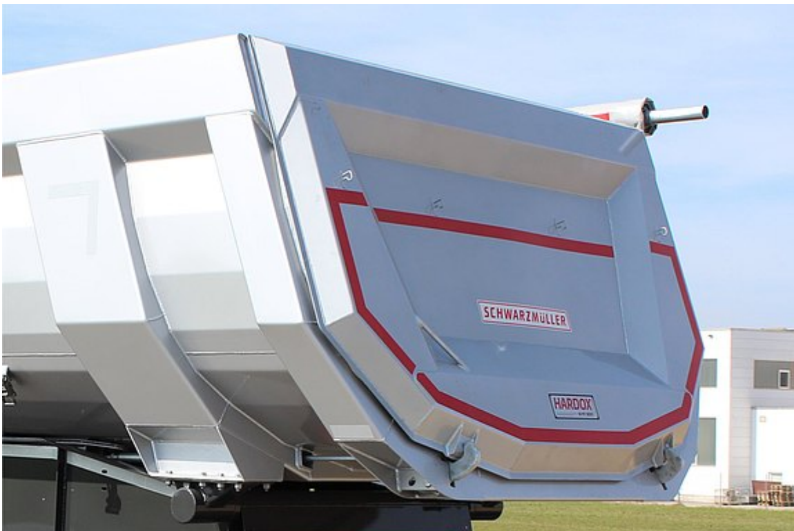
OPTIONAL: External rear wall for higher load volume
