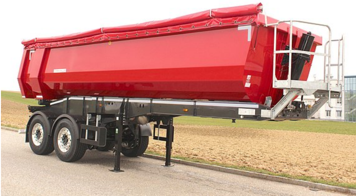
2-axle aluminium segment tipper semitrailer
