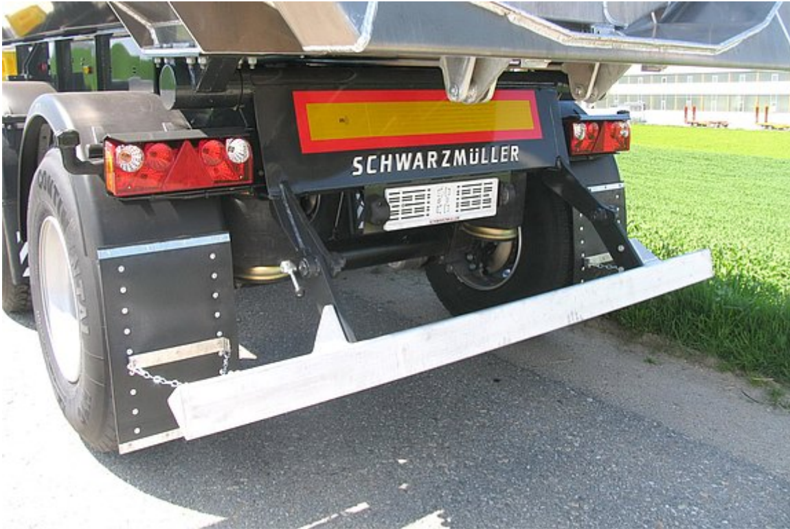
Foldable aluminium trapezoidal underride protection
