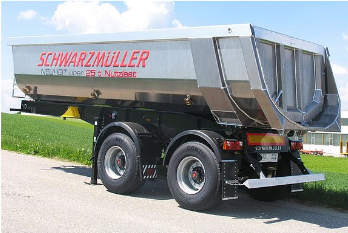
2-axle aluminium segment tipper semitrailer - wheelbase 1,810 mm
