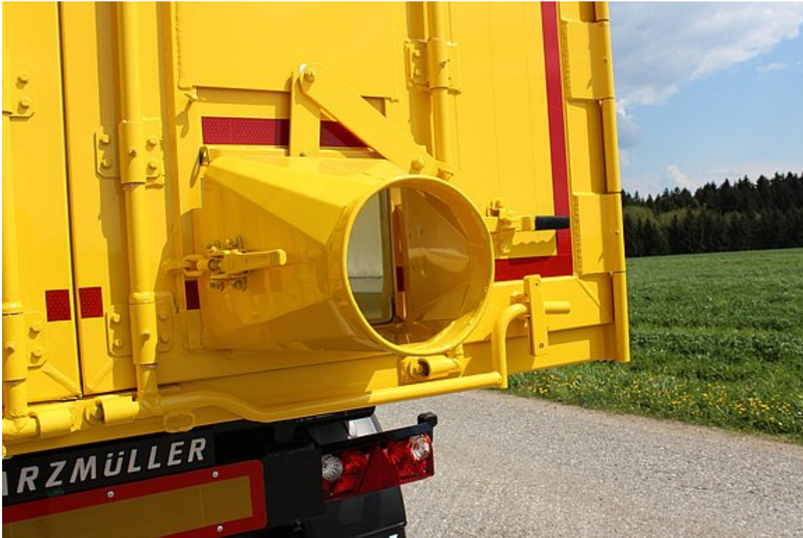
OPTIONAL: a discharge funnel incl. bracket on chassis - suitable for grain feeder
