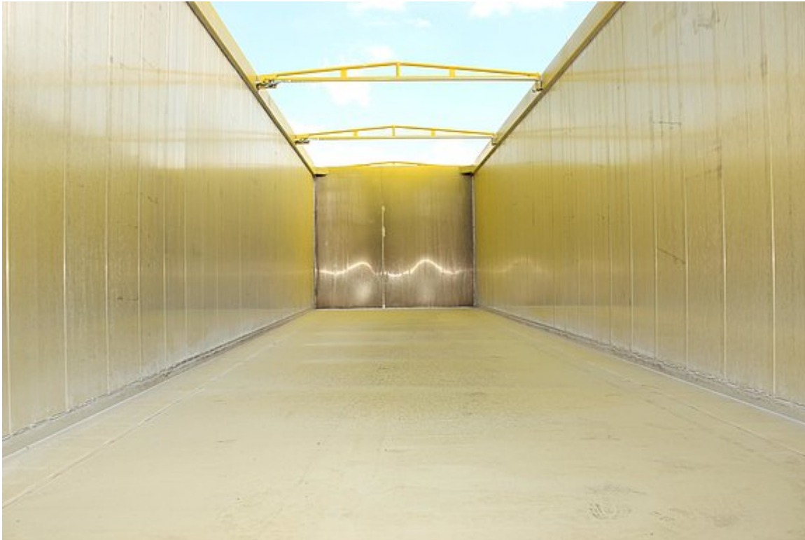
High-grade aluminium tipper made of hollow profiles, for ideal protection against impacts and wear
