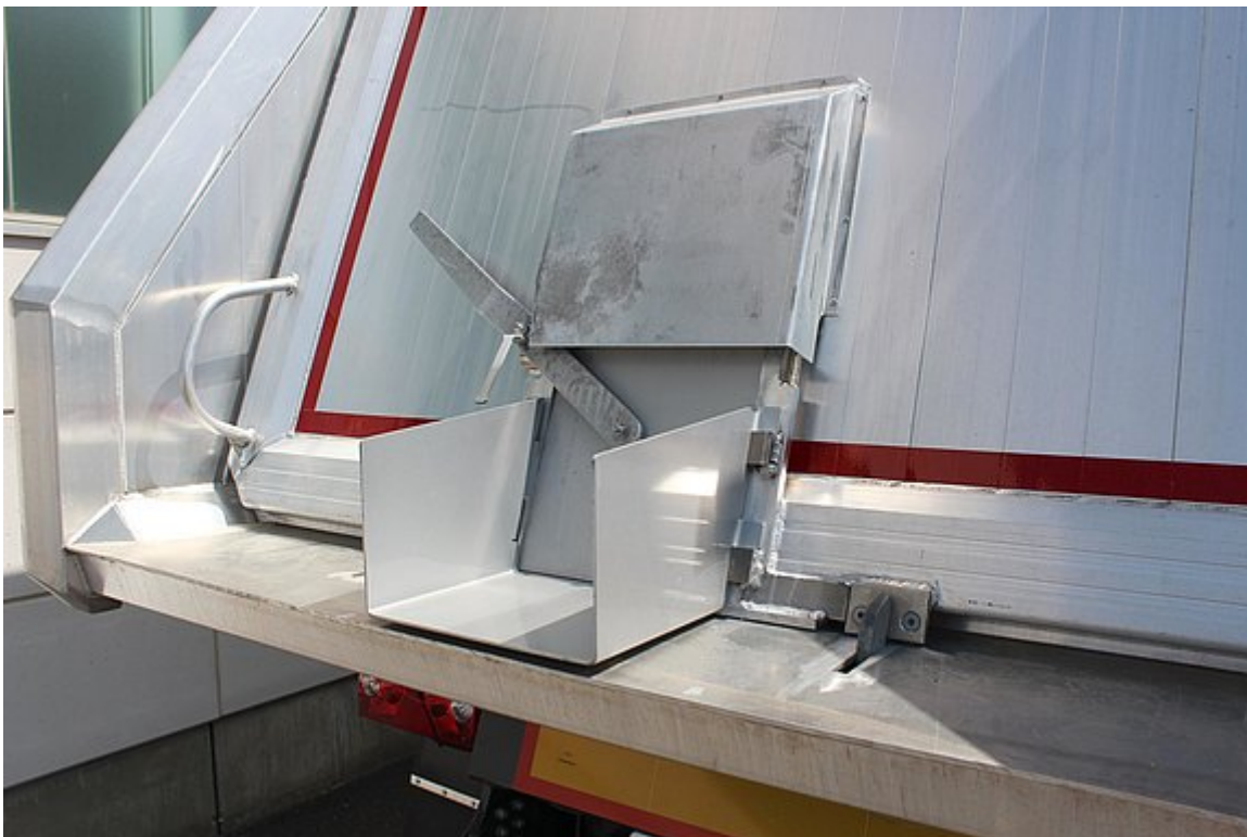
OPTIONAL: Grain feeder with dosing lever and removable discharge funnel in hinged rear wall
