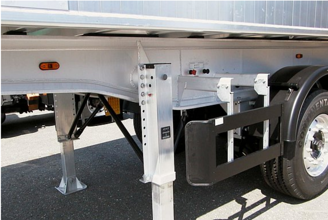
Stable and torsionally rigid aluminium chassis design with additional torsion tubes for considerable payload advantage
