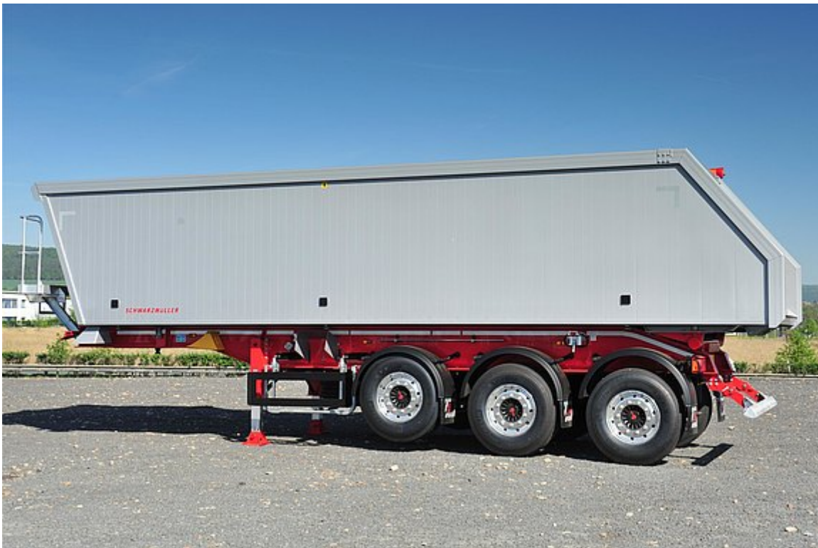
3-axle full aluminium hollow profile tipper semitrailer
