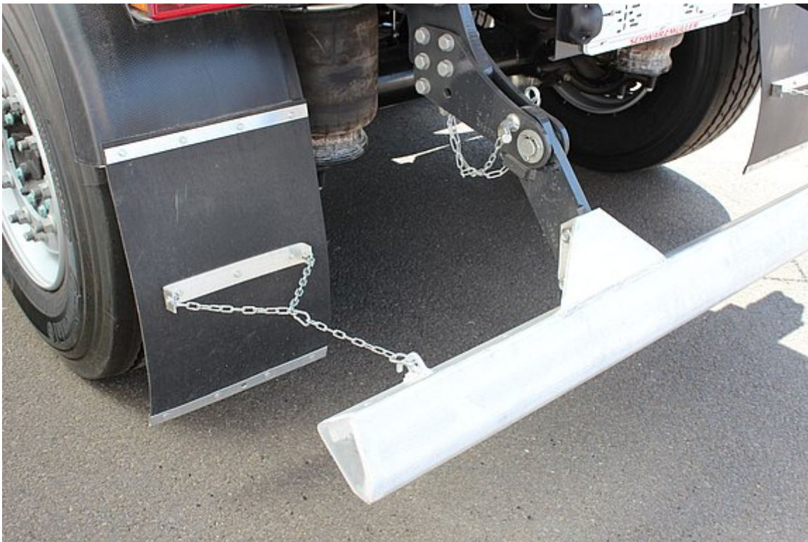
Foldable aluminium trapezoidal underride protection
