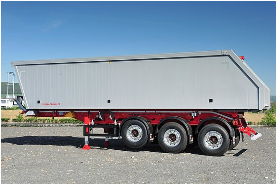
3-axle full aluminium hollow profile tipper semitrailer
