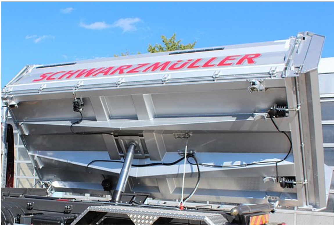
Conical trapezoidal profile side members in high-strength, lightweight design with small bottom
