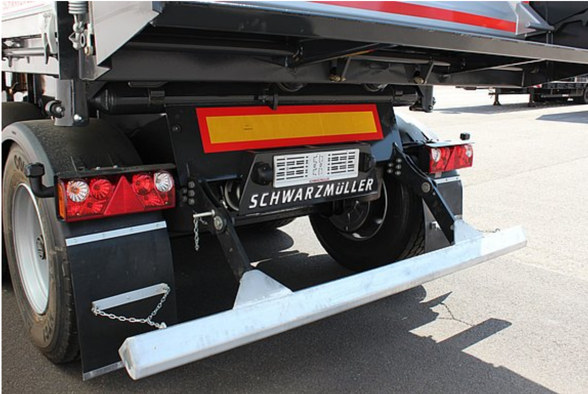
Foldable underride protection for road-finishing use
