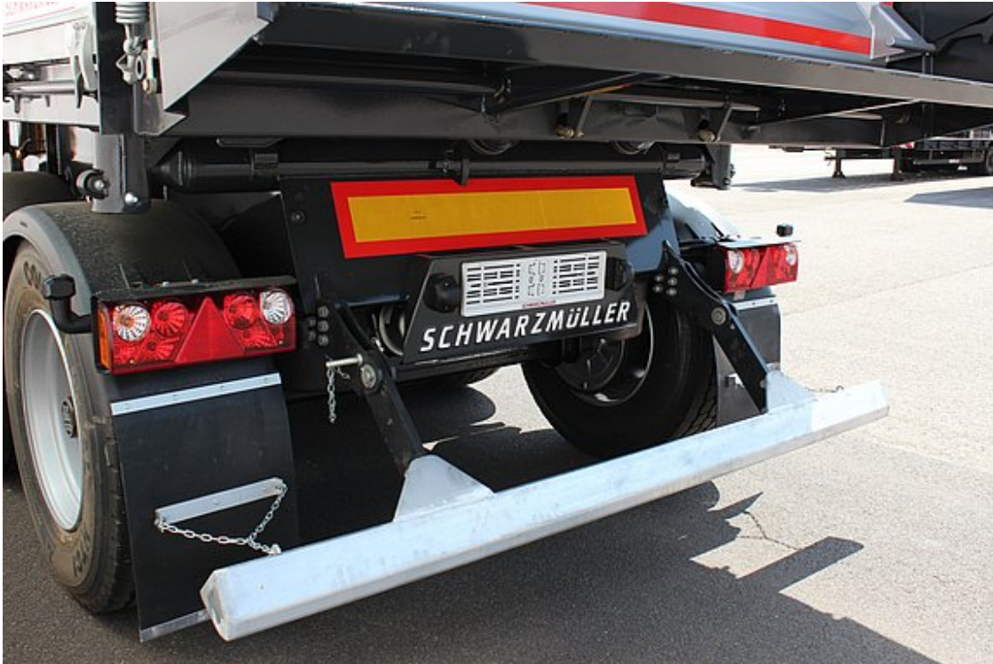
Foldable underride protection for road-finishing use
