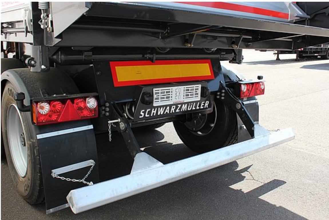
Foldable underride protection for road-finishing use
