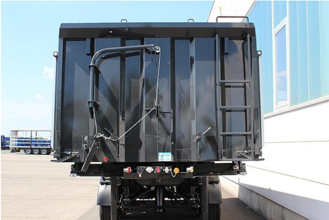
Fixed steel sheet front wall with lashing eyes, ladder and retaining brackets
