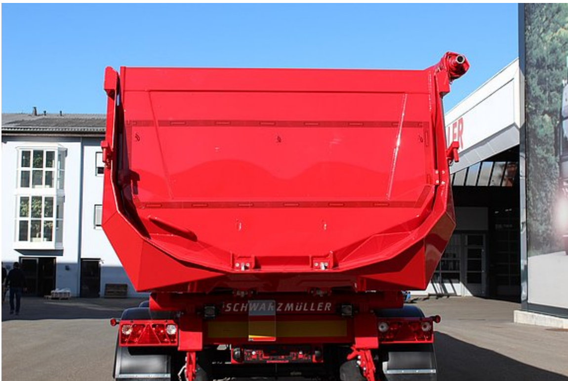
Insulated rear wall = hinged wall with recessed bearing and autom. mech. 2-hook central locking
