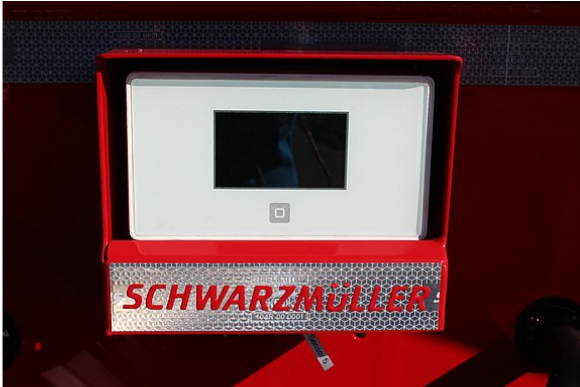
Temperature analysis unit in a sturdy box
