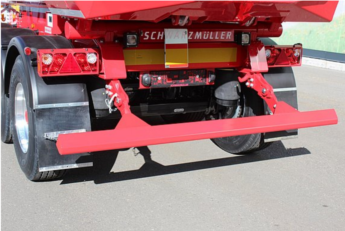
Folding aluminium trapezoidal underride protection, can be folded up pneumatically as an option
