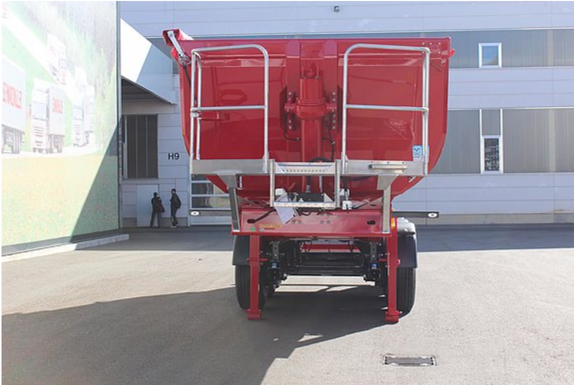
Insulated front wall with hard chrome-plated, high-grade front tilt cylinder
