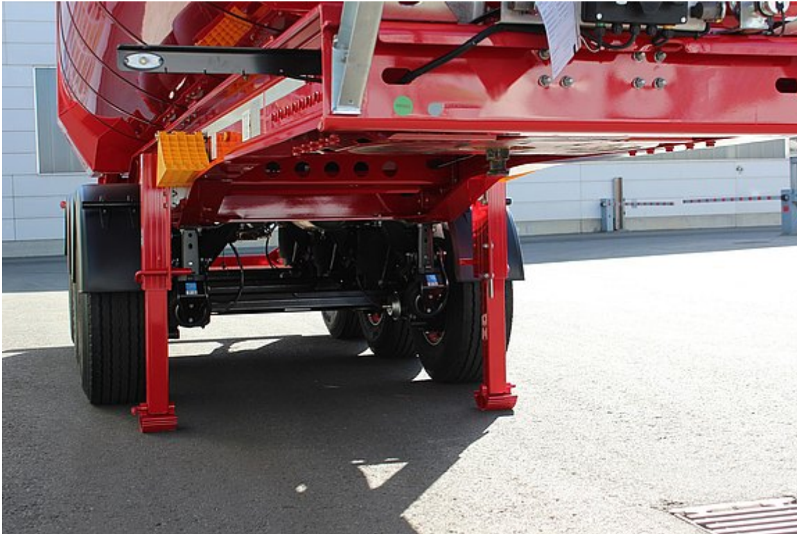
Stable, torsionally rigid aluminium chassis design with additional torsion tubes for high tipping stability
