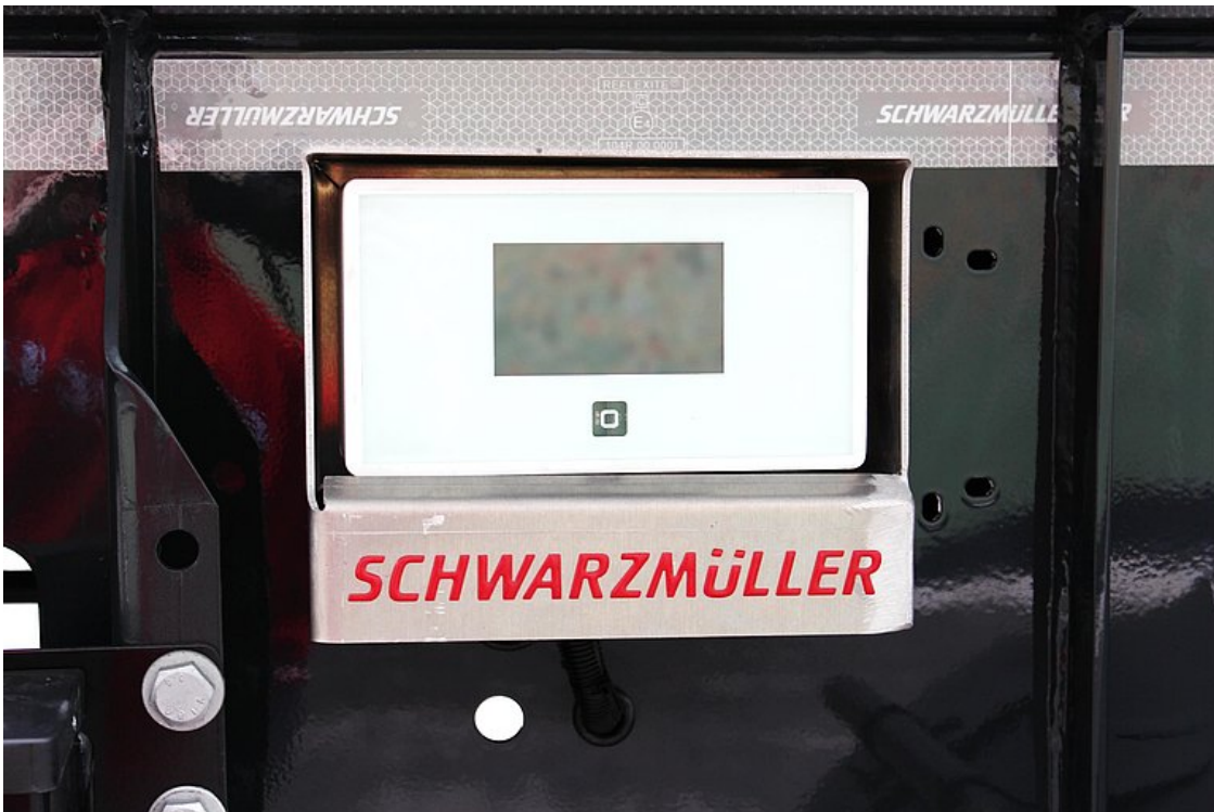
Temperature analysis unit in a sturdy box
