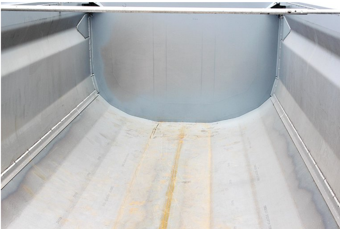
Continuous 3 mm steel wear floor, with welded aluminium frame
