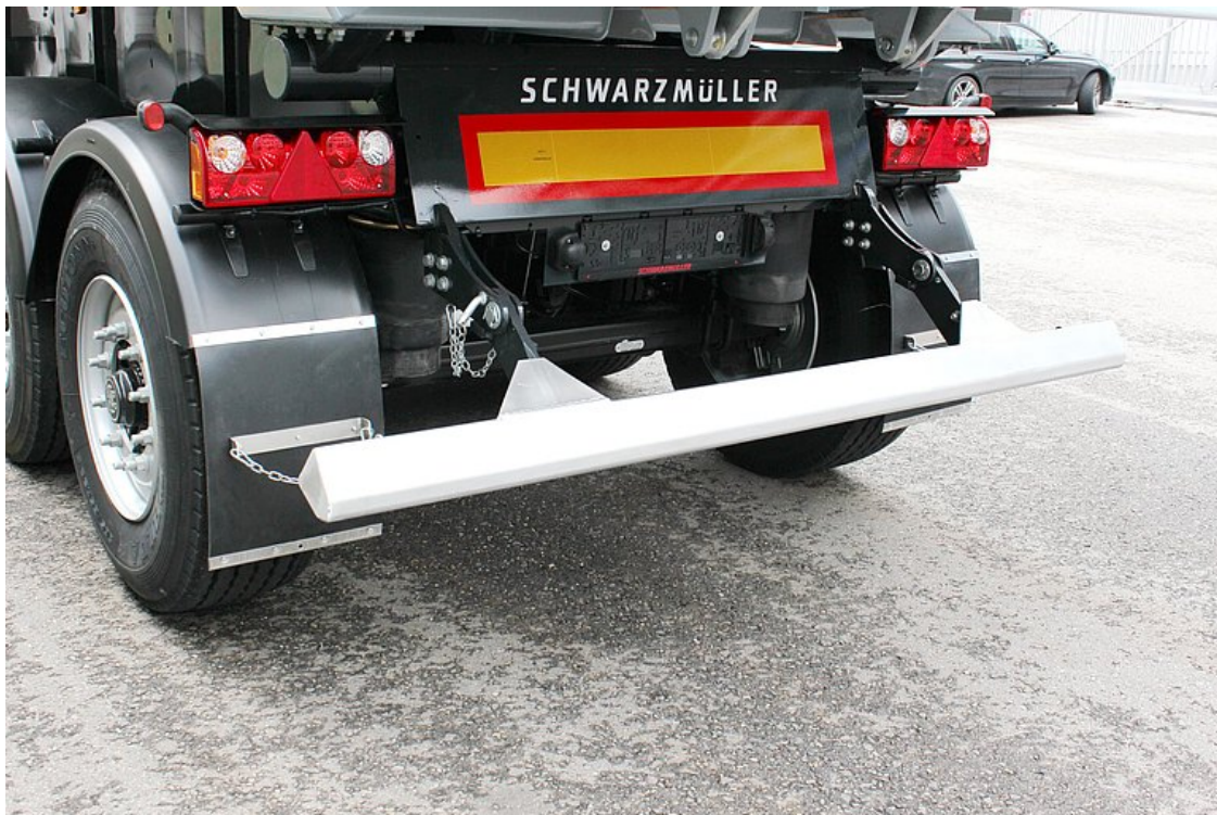
Folding aluminium trapezoidal underride protection, can be folded up pneumatically as an option
