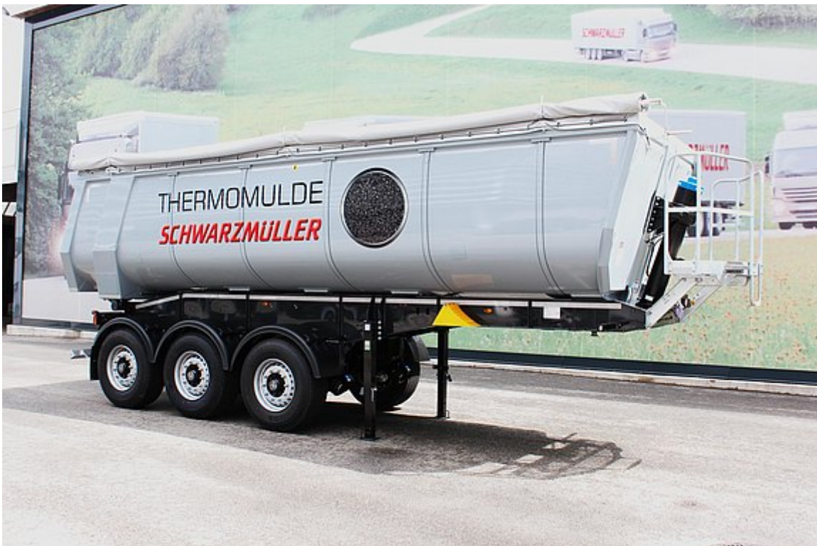
Stable, torsionally rigid Naxtra chassis design with additional torsion tubes for high tipping stability
