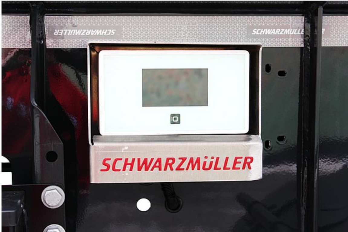
Temperature analysis unit in a sturdy box
