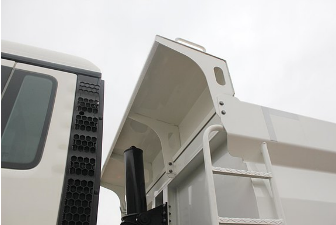
Front wall at top with raised excavator protection
