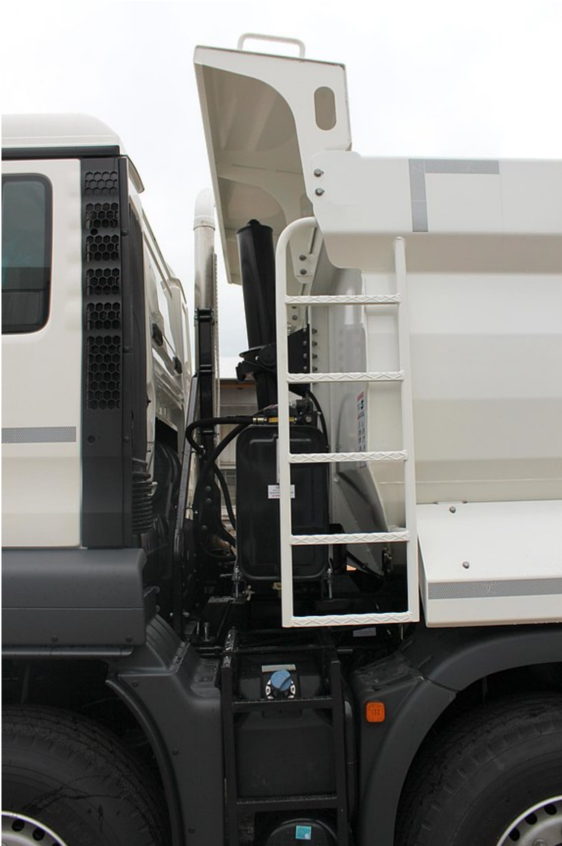
Fixed ladder on outside front left side
