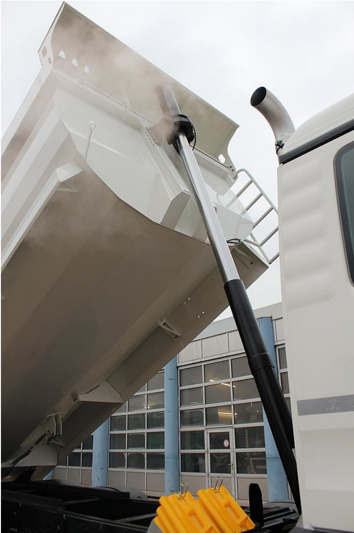
Hard chrome-plated, high-quality front tilt cylinder
