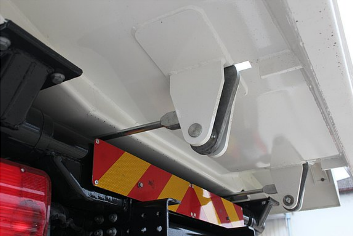
Automatic mechanical rear wall locking
