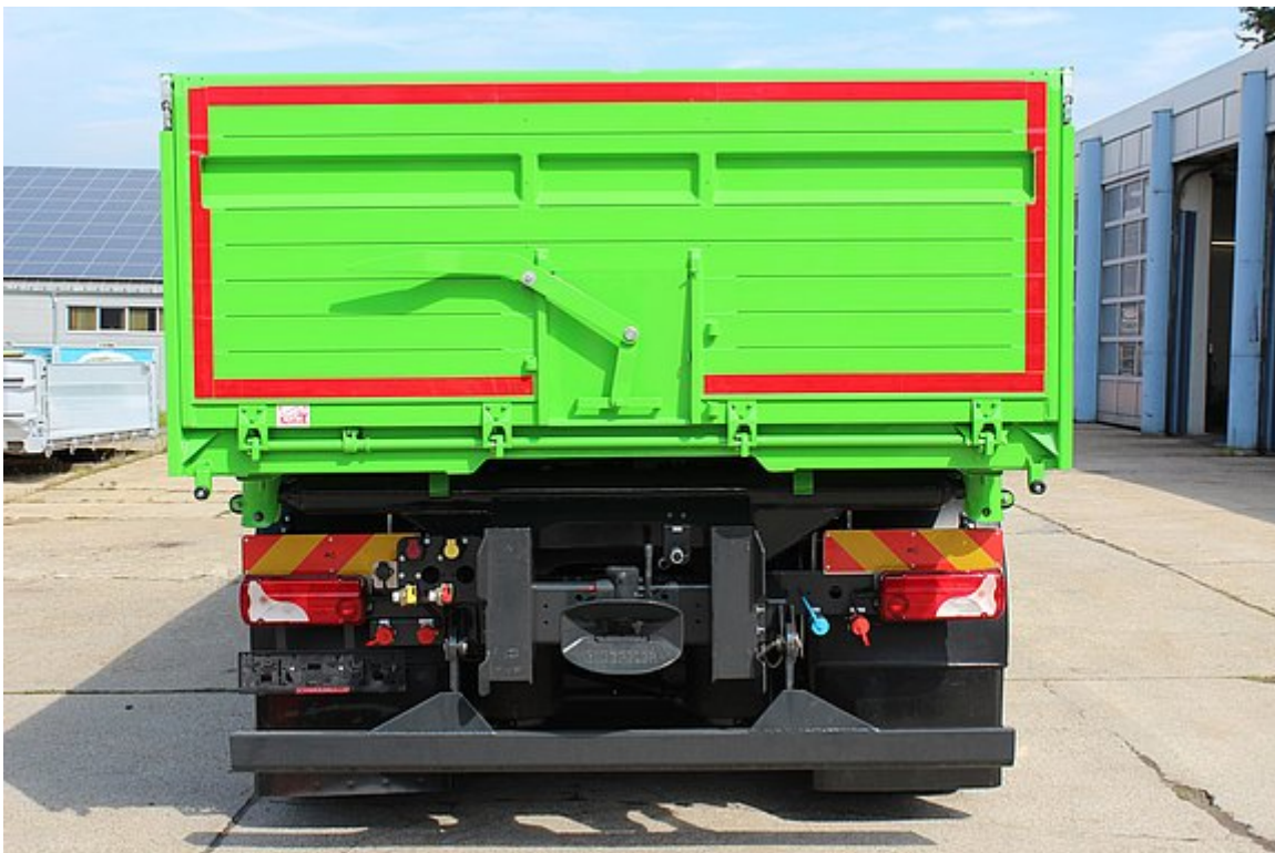
Aluminium hollow profile rear wall and additional option with grain feeder approx. 400/400 mm with side-mounted dosing lever
