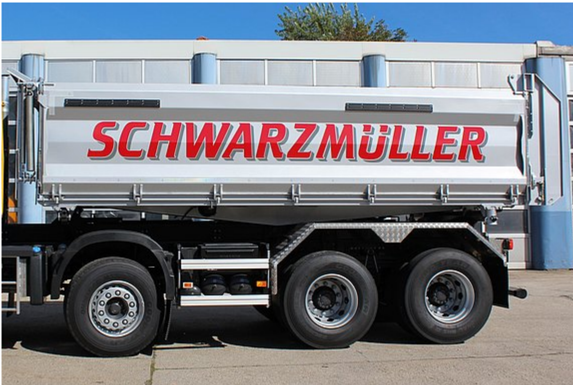
OPTIONAL: Reinforced side walls with material-repellent membrane construction made from fine-grained special steel panels
