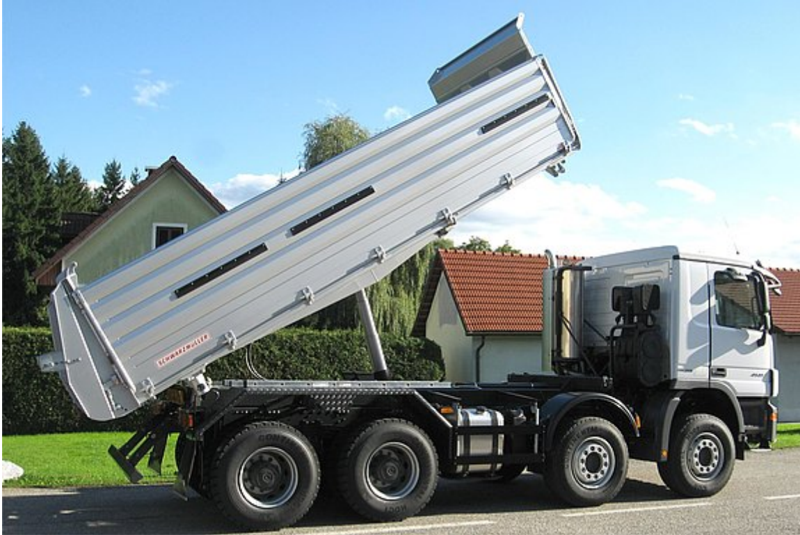
3-way tipper body on 4-axle truck - building site
