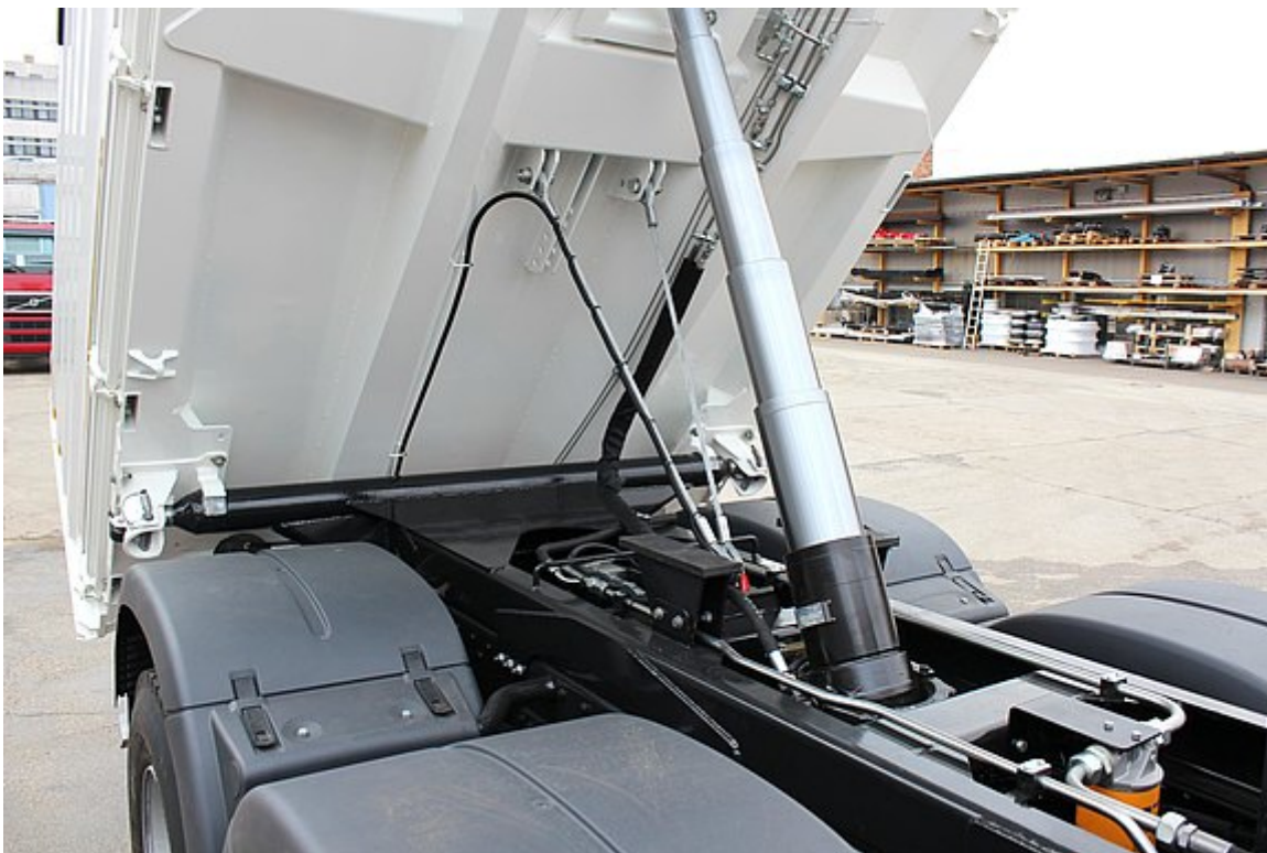
Hard chrome-plated, high-quality tilt cylinder
