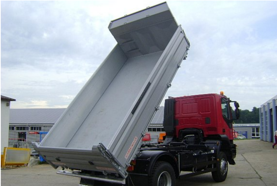
3-way tipper body on 2-axle truck - building site
