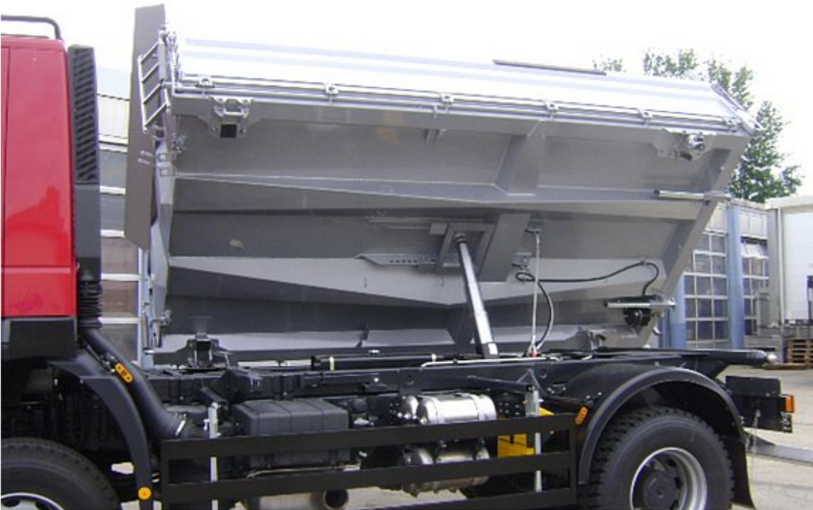
Tipper body design with conical trapezoidal profile side members in high-strength, lightweight design with small bottom panels for high dent resistance and shock absorption
