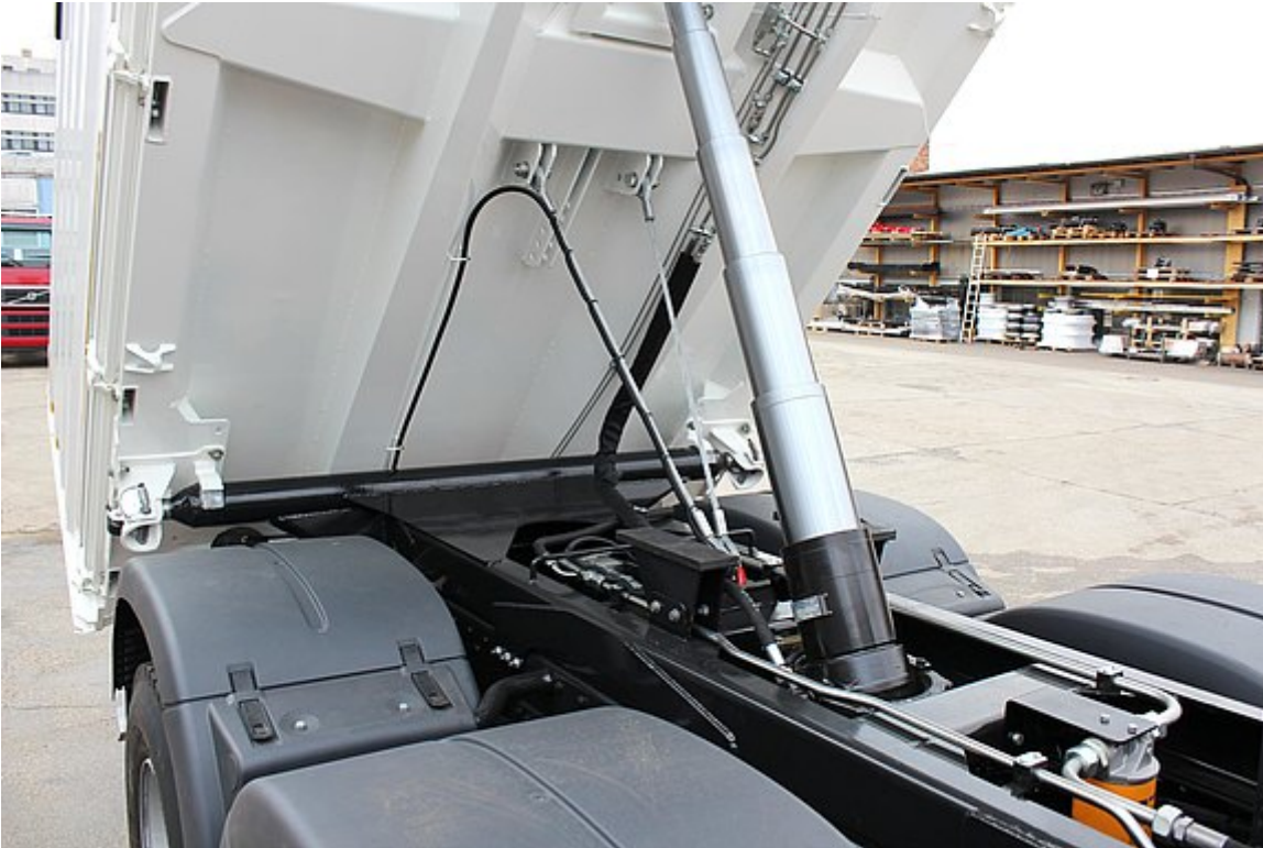
Hard chrome-plated, high-quality tilt cylinder
