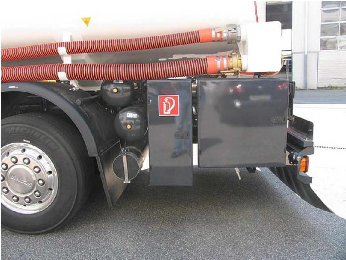
Separate aluminium boxes on the left and right for dipstick operation with a small spirit level
