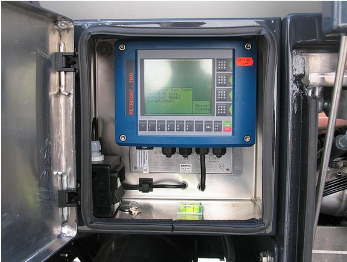
Separate aluminium boxes on the left and right for dipstick operation with a small spirit level
