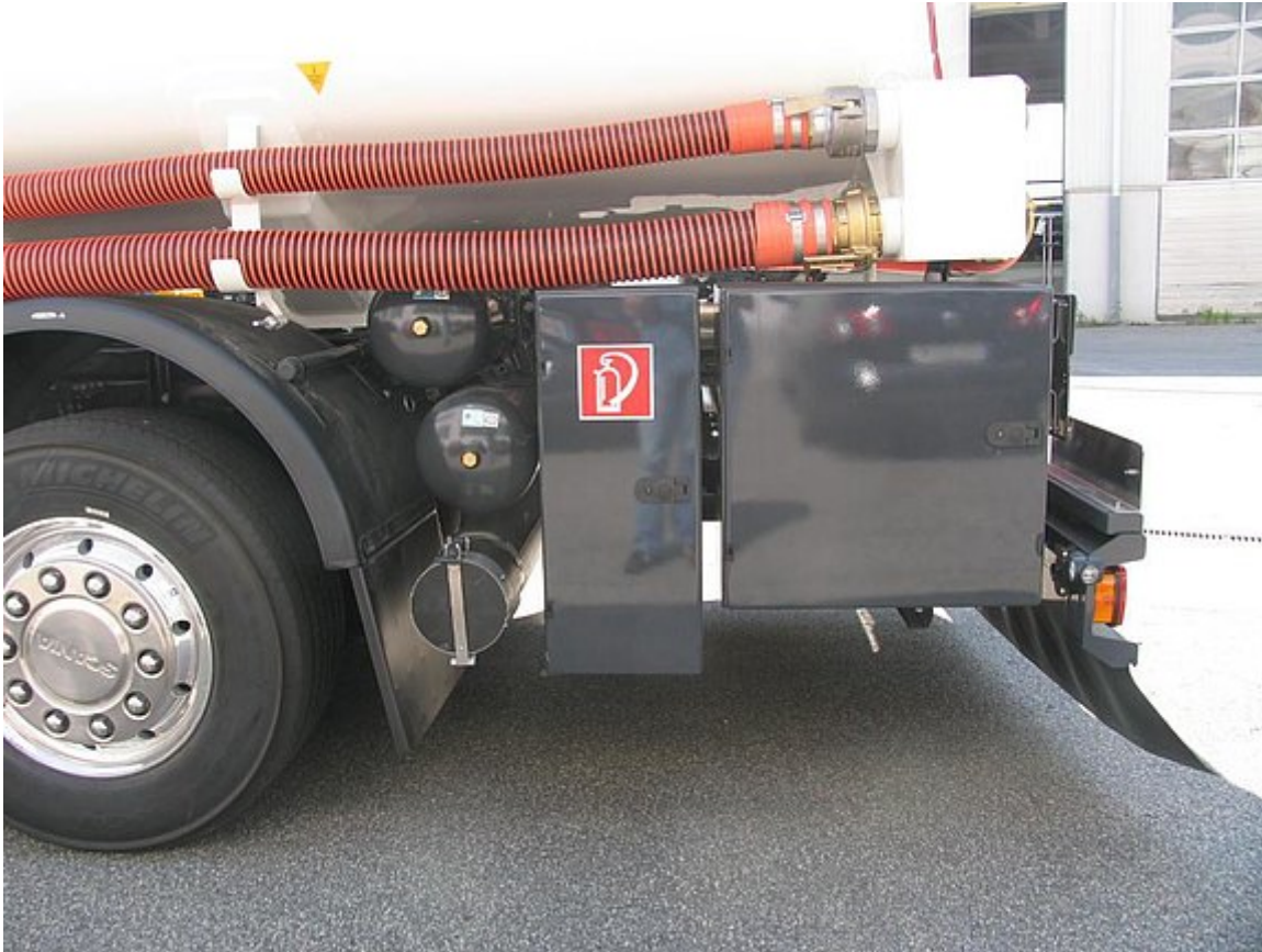
Aluminium box for 12 kg fire extinguisher and accessories box
