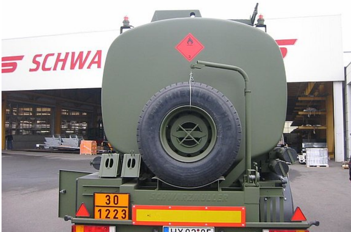
Ideal arrangement of spare wheel at the rear of the vehicle
