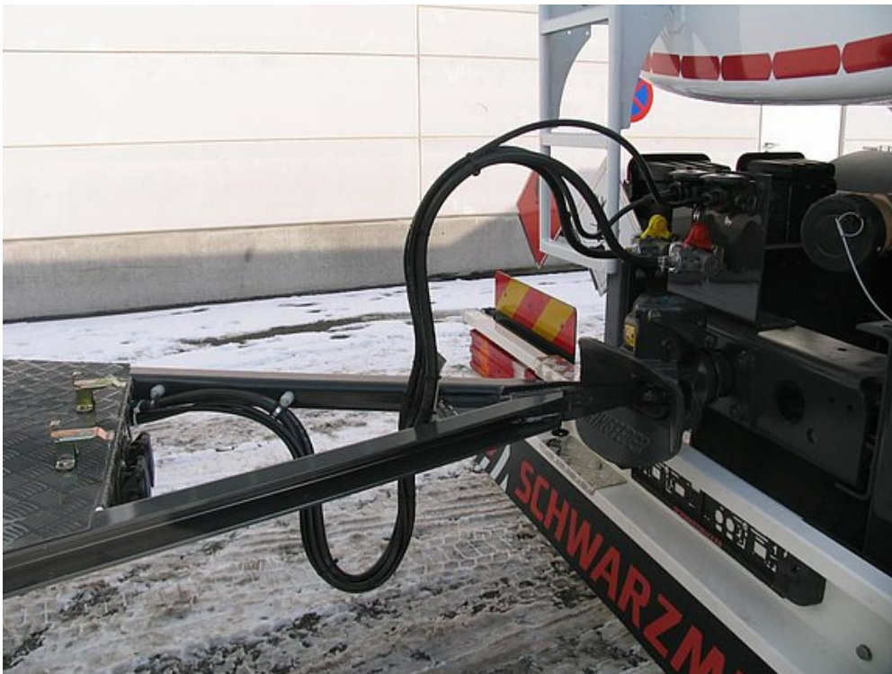
Drawbar with connection cables to the truck
