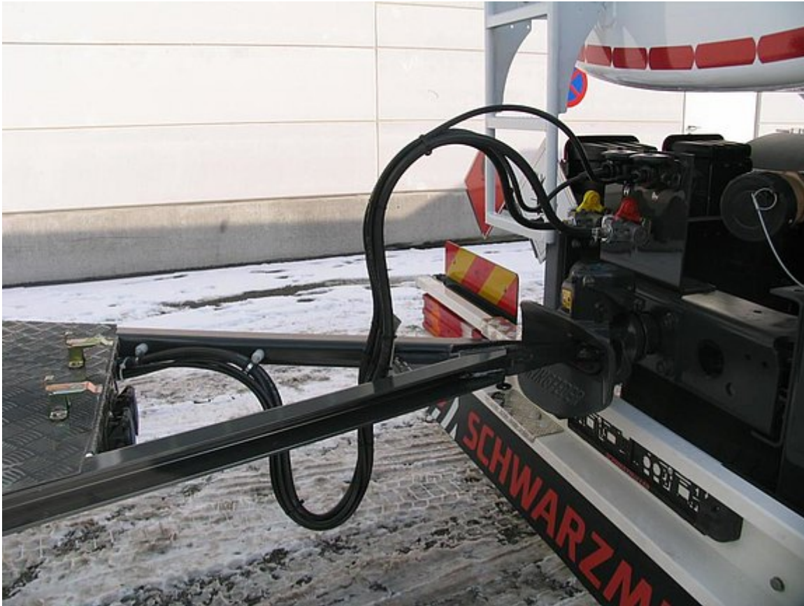
Drawbar with connection cables to the truck
