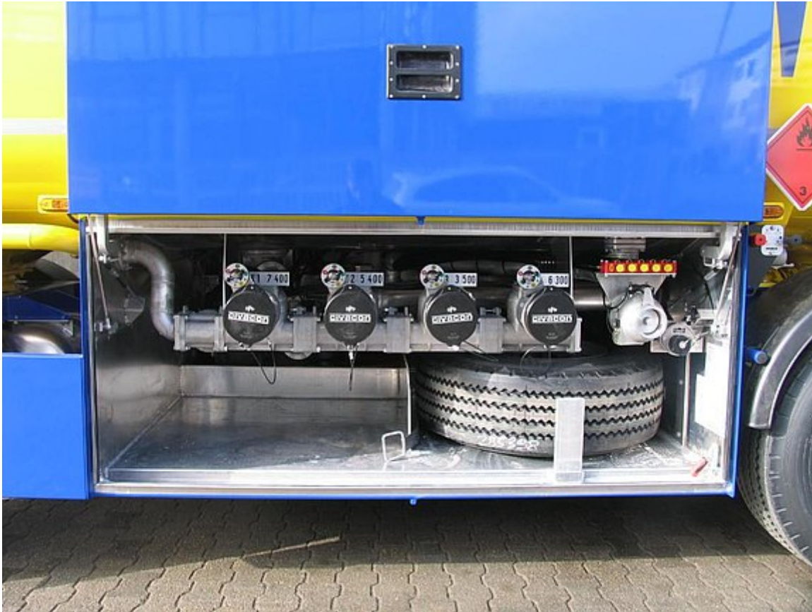
Fittings cabinet with parallel sliding cabinet doors and storage option for spare wheel
