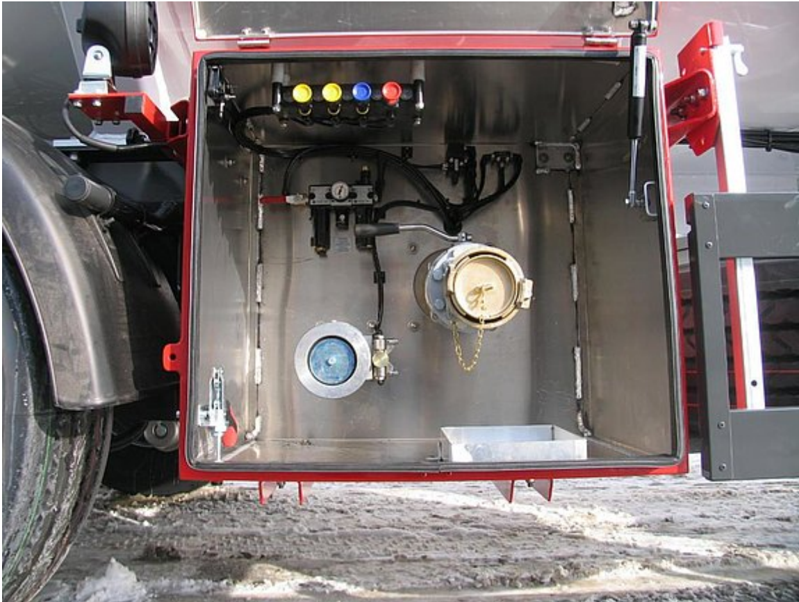
Discharge box with upward-opening door to protect the fittings
