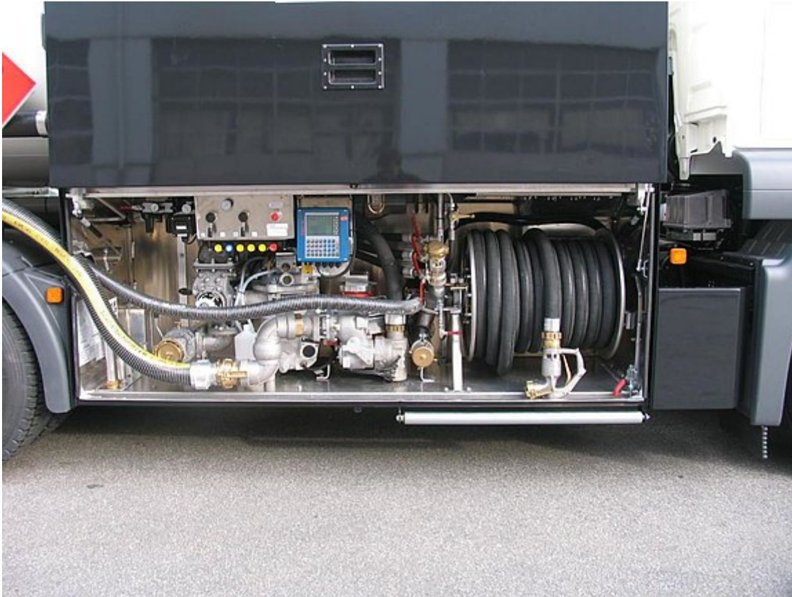
Fittings cabinet with parallel sliding cabinet door
