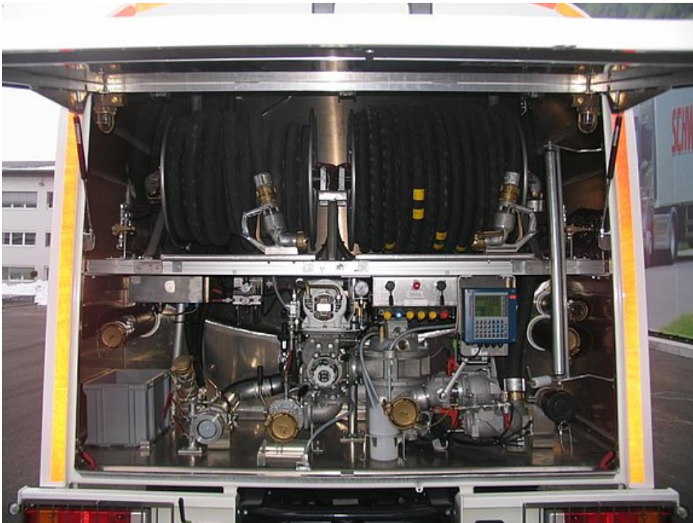
Rear-mounted cabinet with folding door for measuring systems and hose reel
