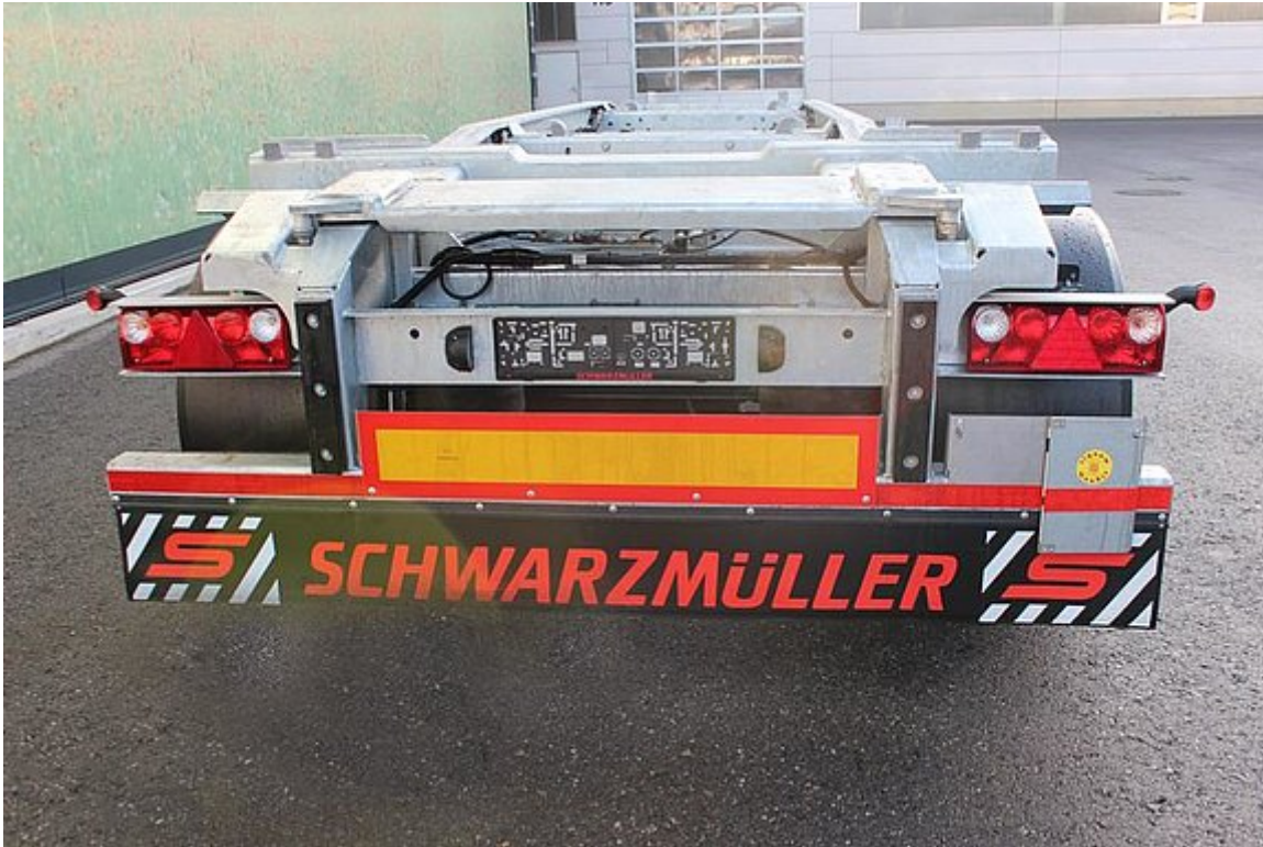
Bolted steel underride protection, with vertical rubber buffers
