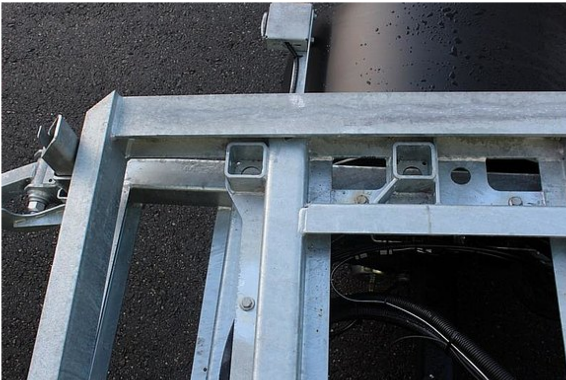
Adjustable stops at front for various container lengths
