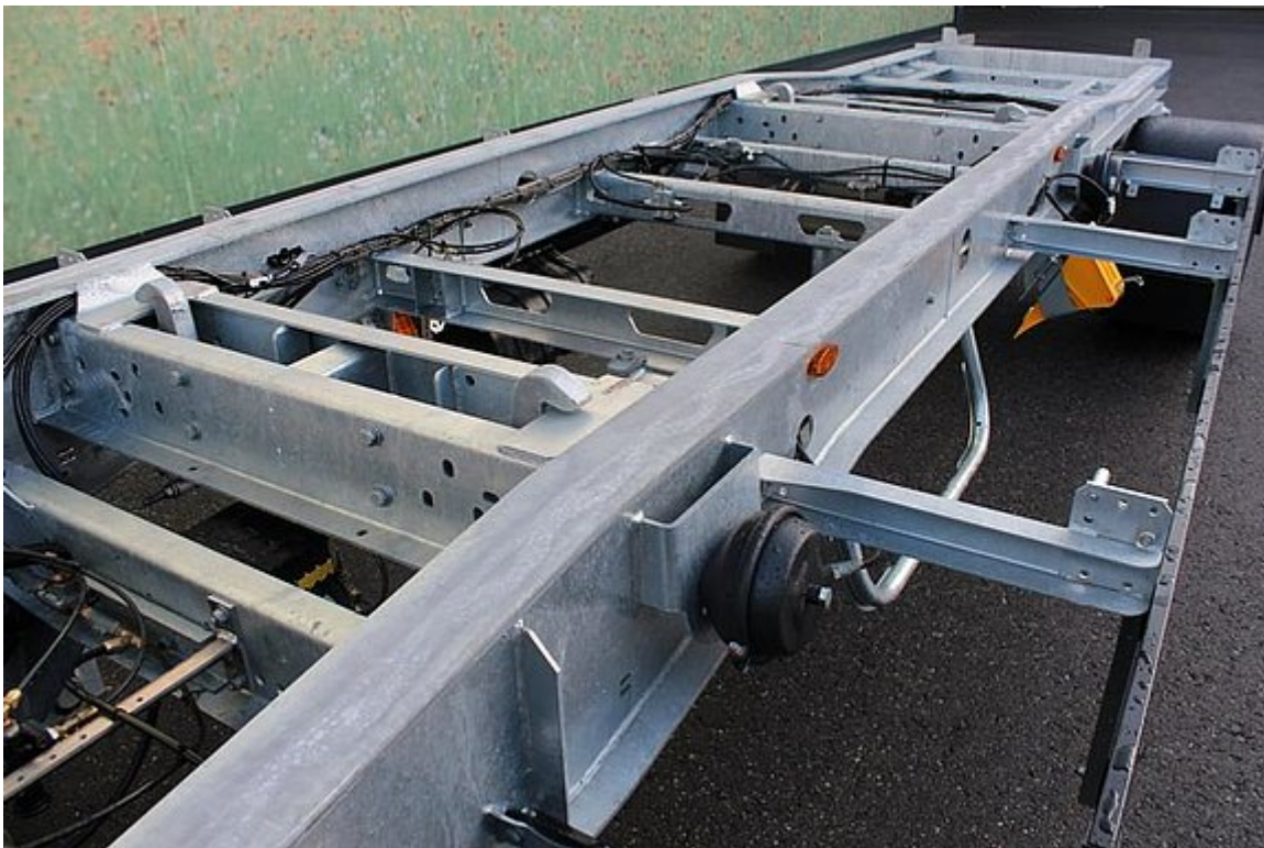
Frame length approx. 7,000 mm for container lengths of 5,000 - 7,000 mm
