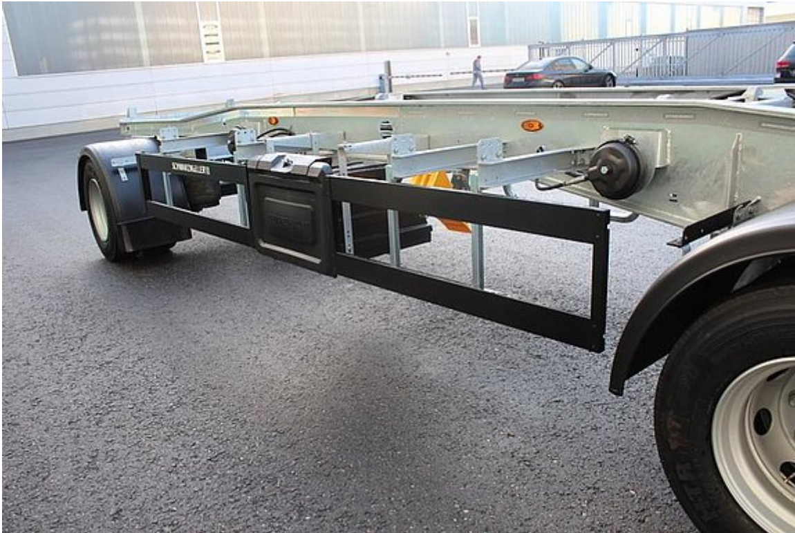
Side collision guard with optional tool kit
