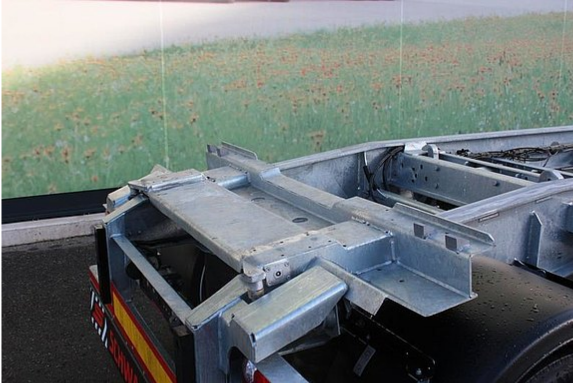
Slide for acceptance of container rollers
