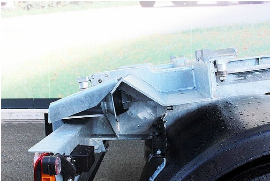
Fixation of slide using rubber buffer
