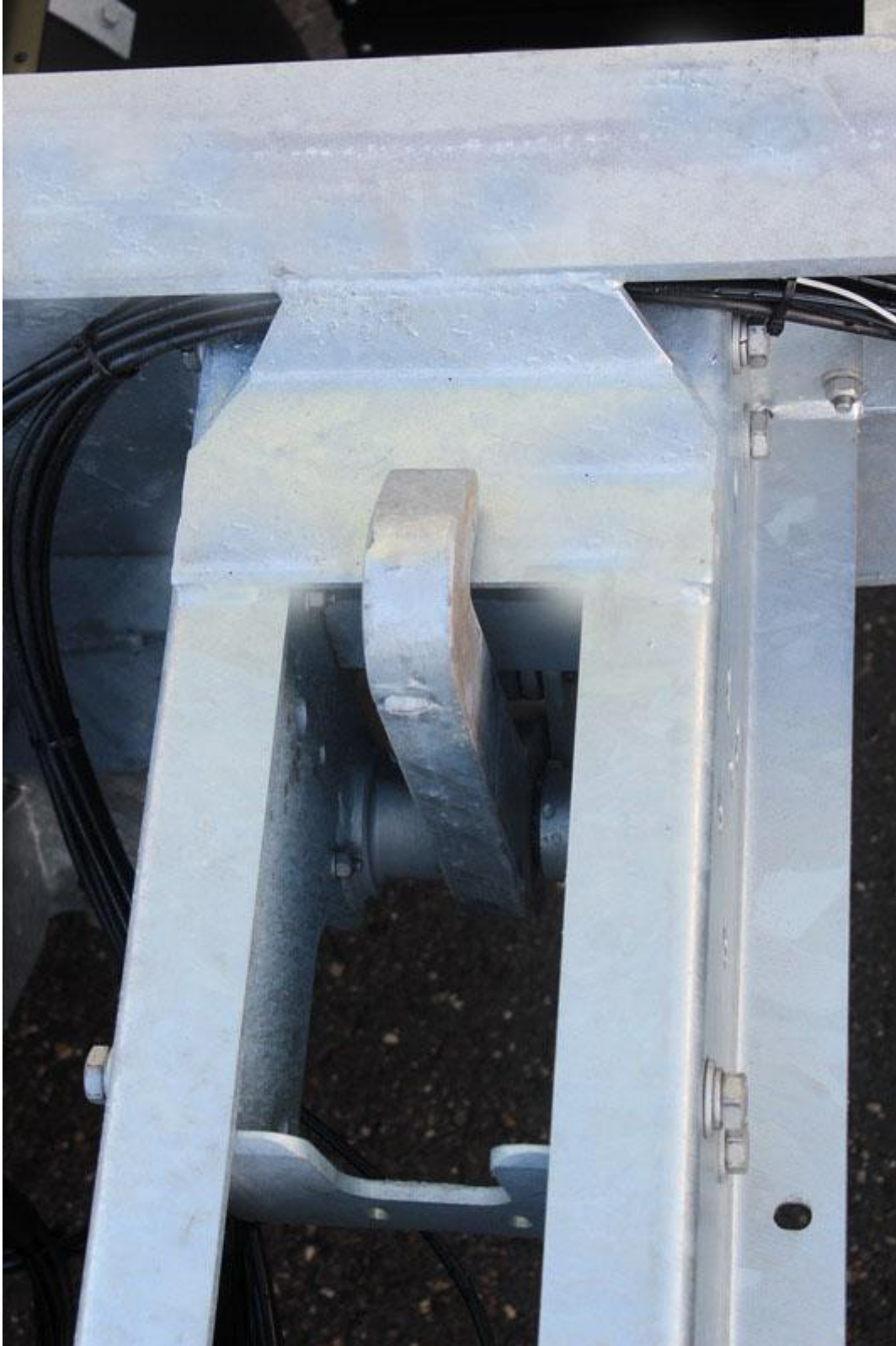
Pneumatic locking hook with switch on trailer
