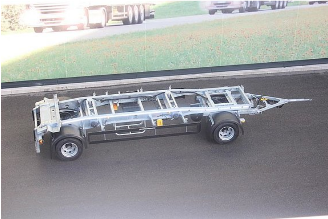
2-axle low-loader swap body trailer chassis for roll-off containers
