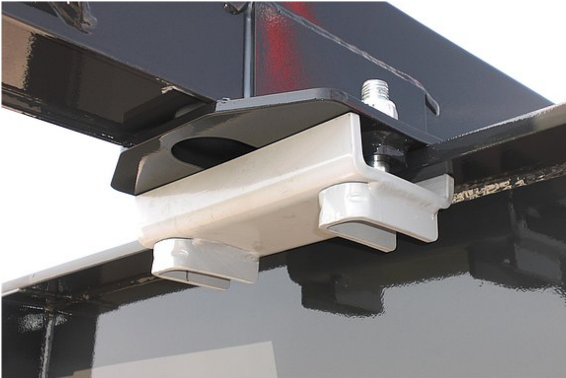
Stanchions mounted via welded clamps = can be moved
