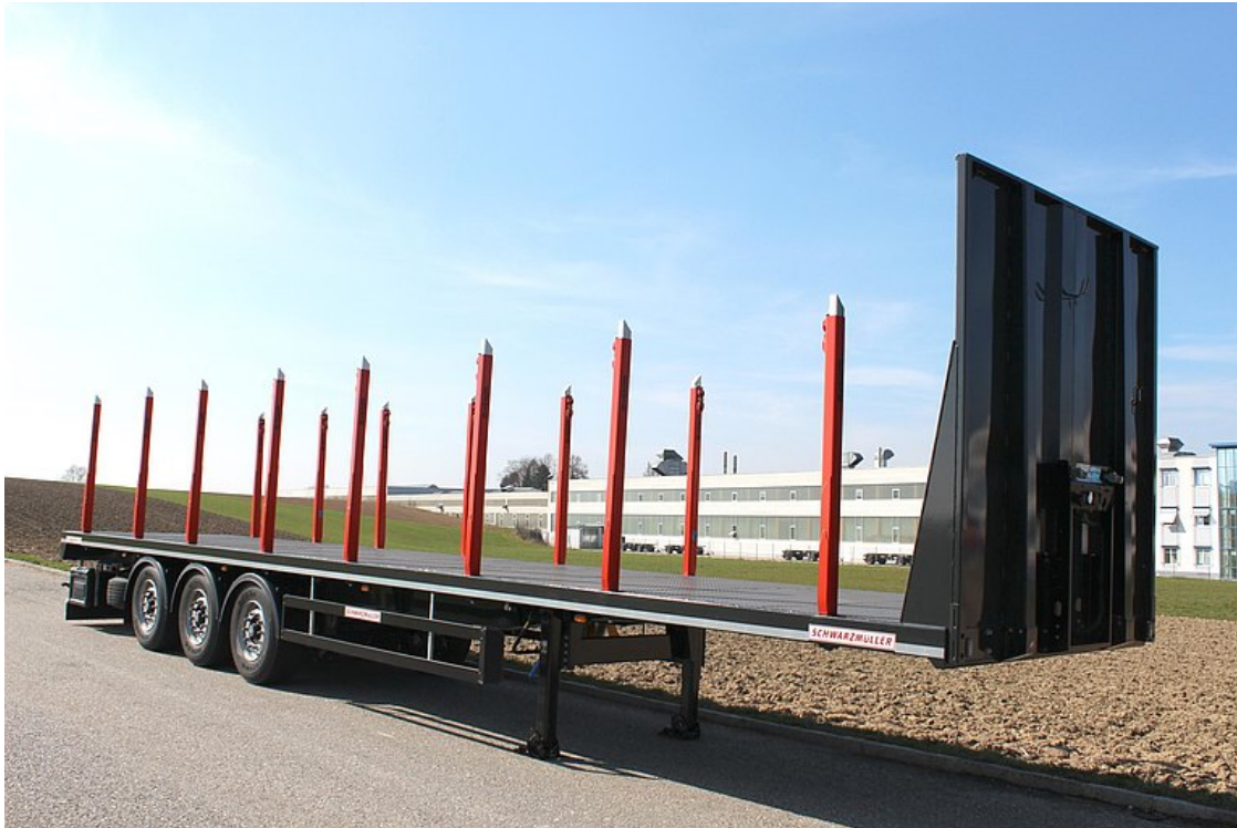
3-axle stanchion platform semitrailer
