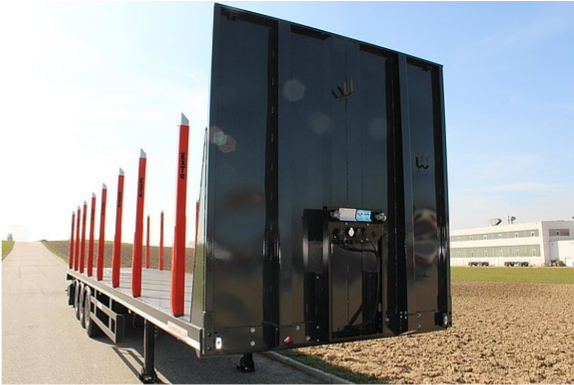
Extra-strong steel profile front wall with centre supports
