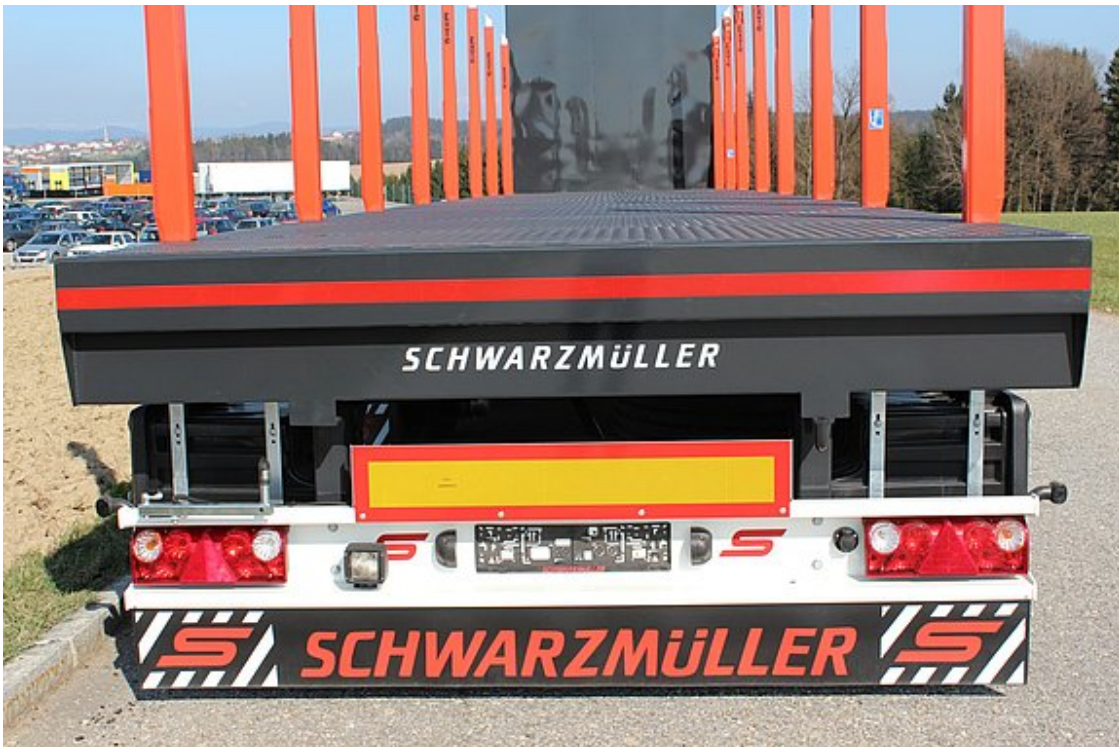
Rear closing element incl. fitted aluminium underride protection
