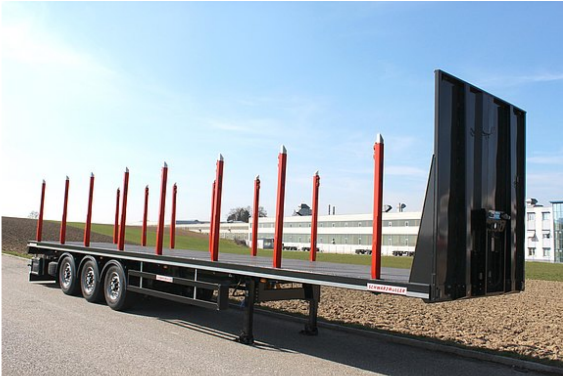
3-axle stanchion platform semitrailer
