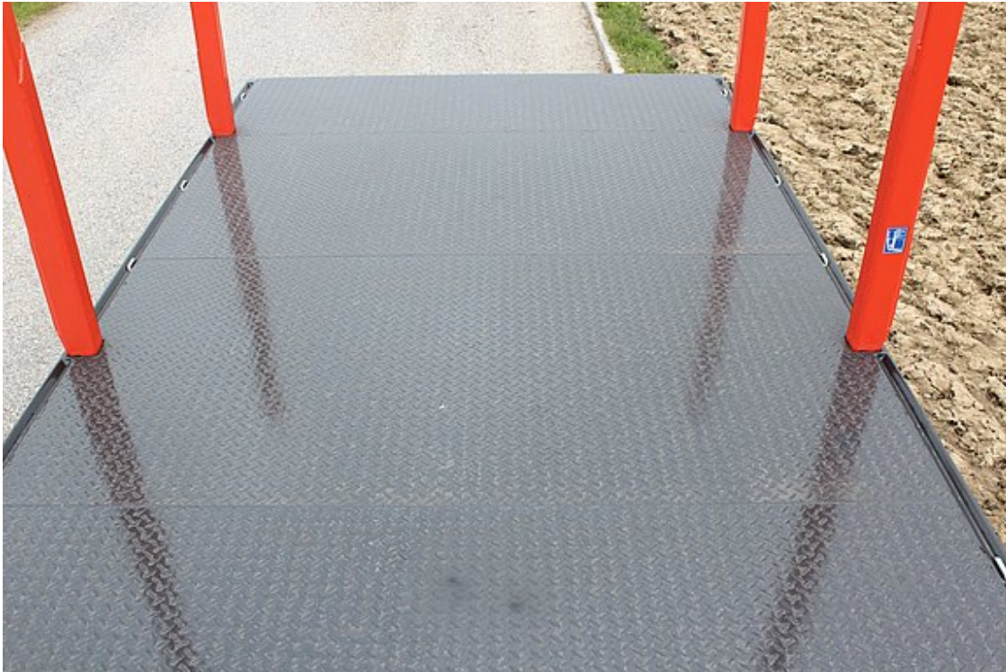
Steel stud plate floor, 5/7 mm, tack-welded
