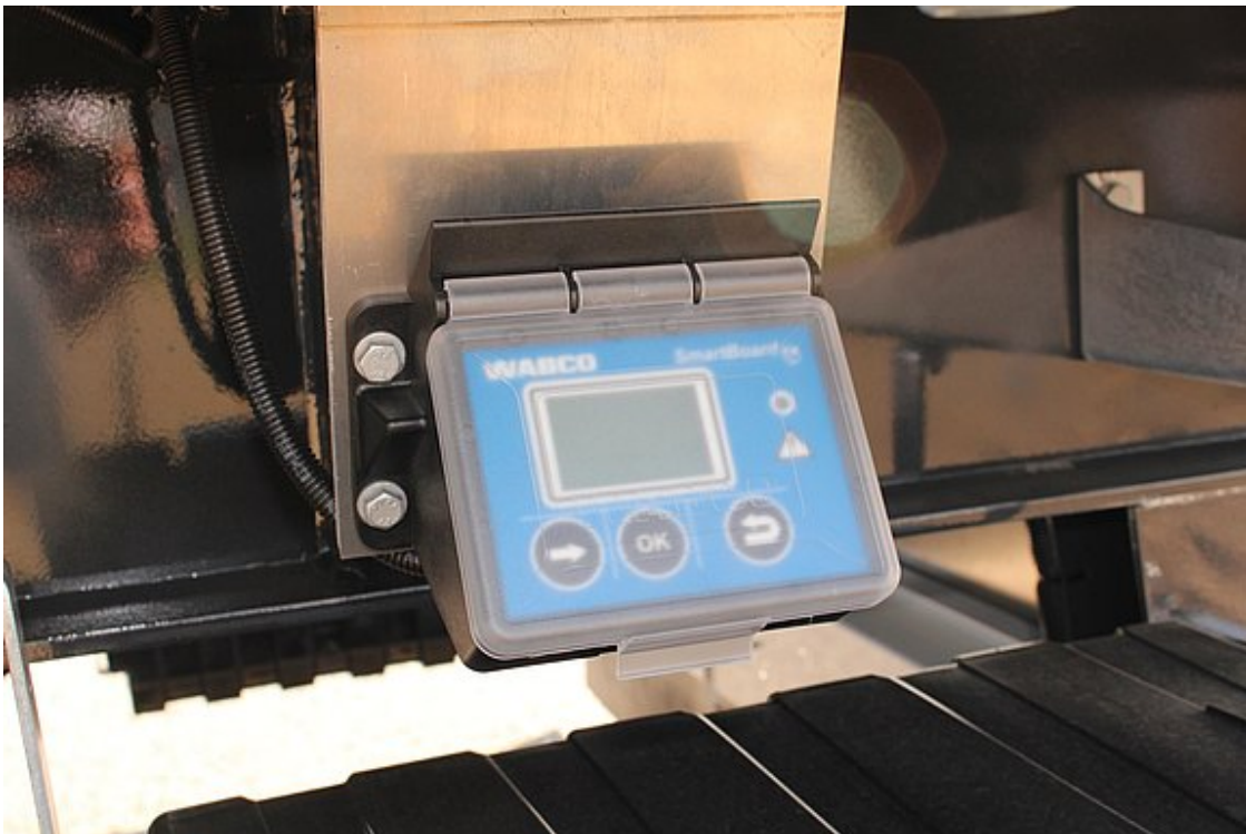
OPTIONAL: SmartBoard for reading data on vehicle display (mileage, axle assembly load, brake diagnostics etc.)
