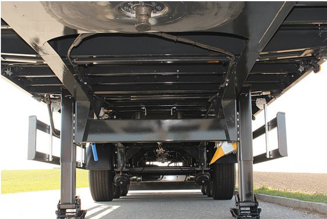
Lightweight frame made from special high-strength NAXTRA steel provides payload advantage of up to 500 kg
