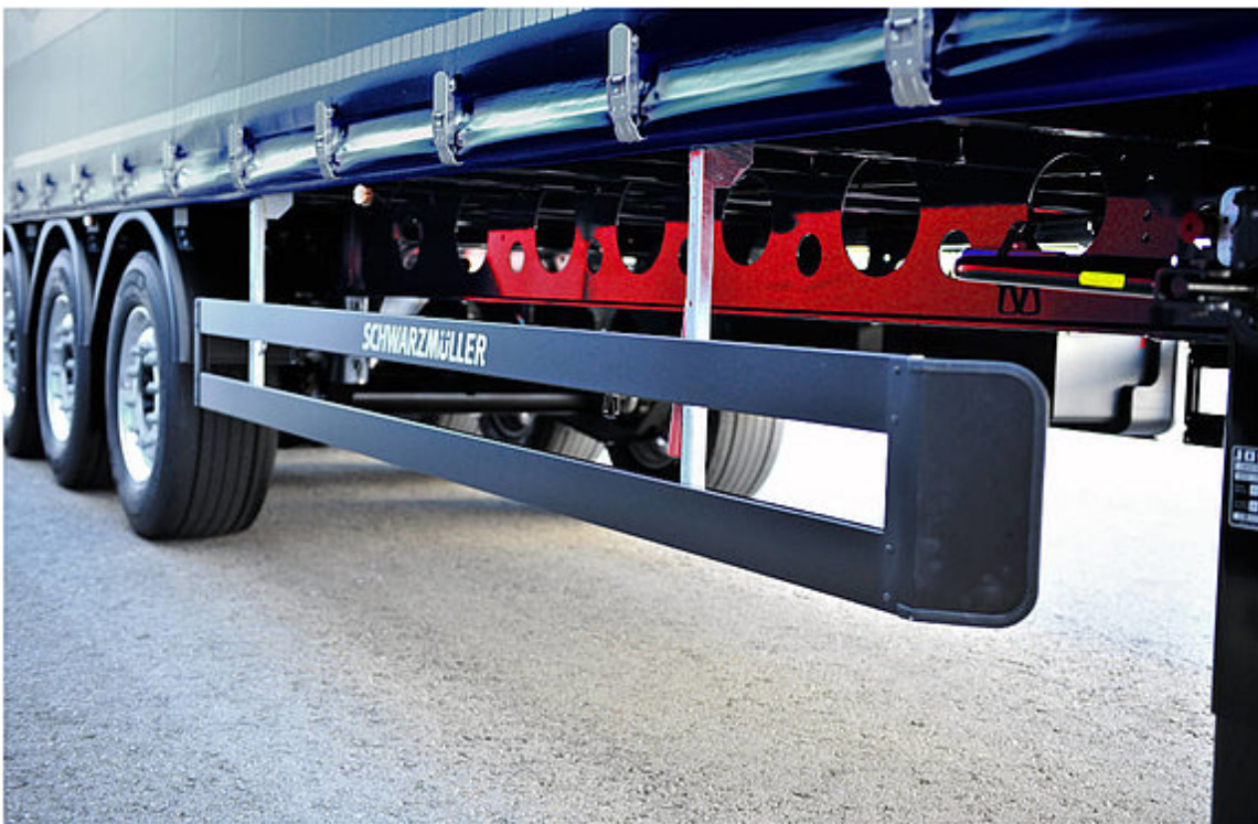
Side impact protection: Statutory cyclist protection to prevent persons from falling down in front of the wheels.
