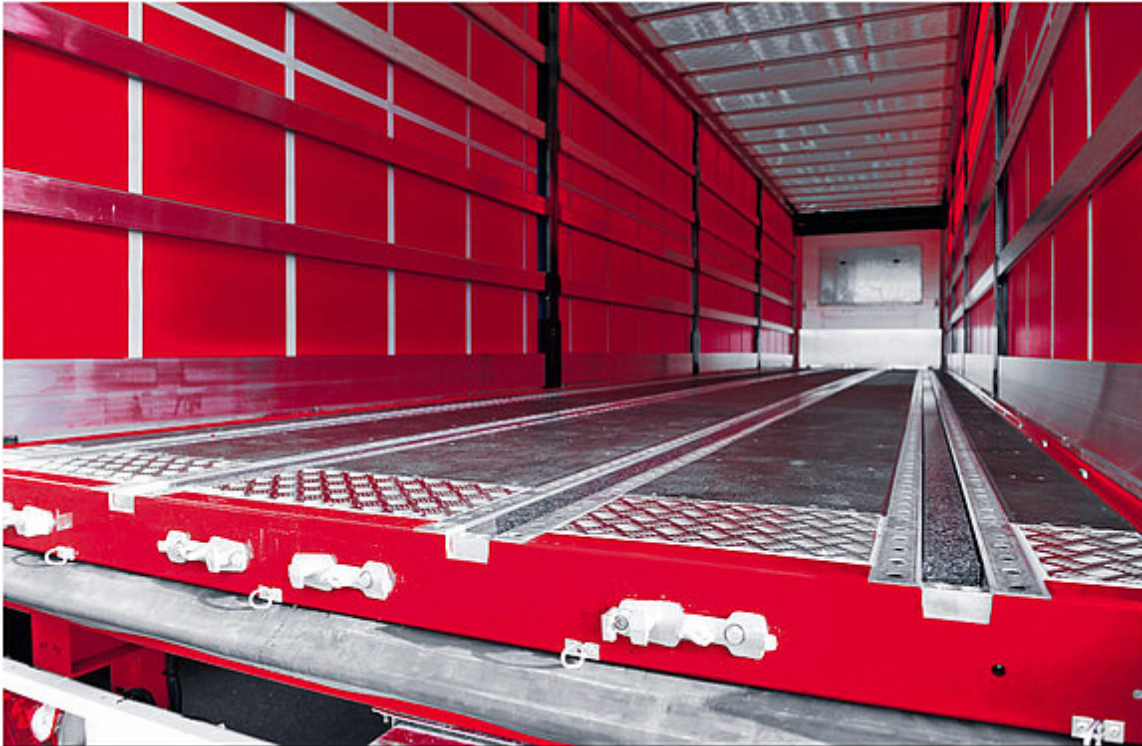
OPTIONAL: Inserts for Joloda rails: In general cargo use, the rails are covered or filled with plastic profile inserts.
