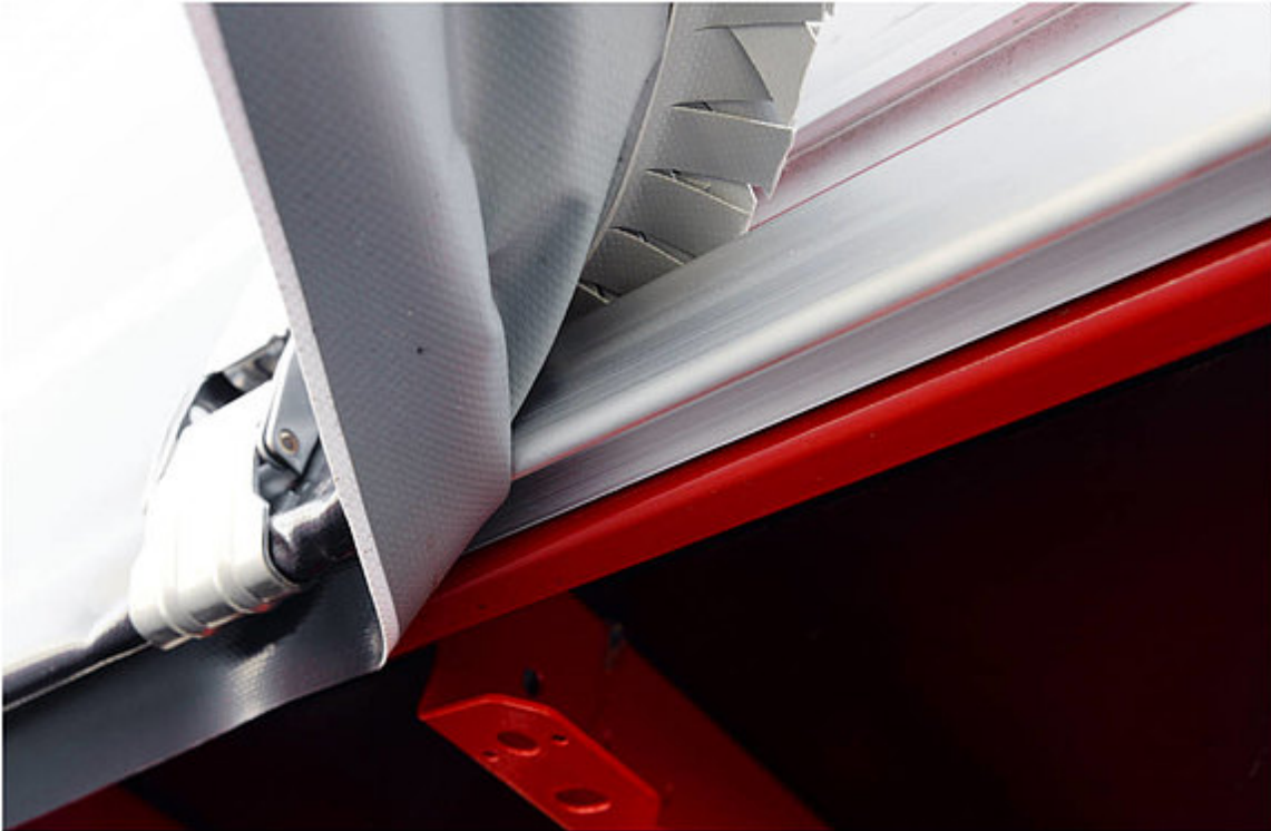
Tarpaulin hooking rack: Vertically attaches the side tarpaulin to the outer frame. Ensures a perfect connection without the tensioners standing aslant.
