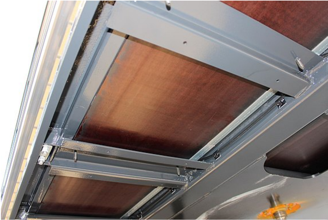
Resin-coated plywood floor, 27 mm, flush with external frame (floor load capacity: 5.460 kg stacker axle load acc. to CSC)
