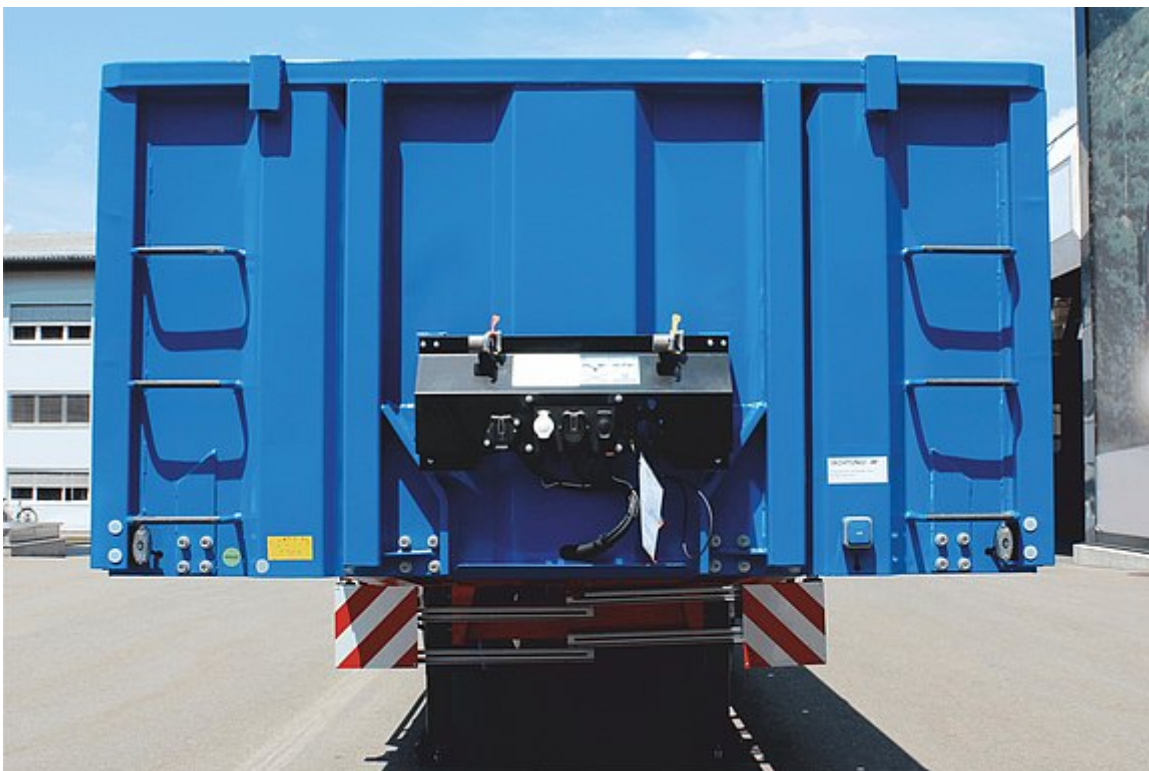
Fixed, reinforced aluminium hollow profile front wall
