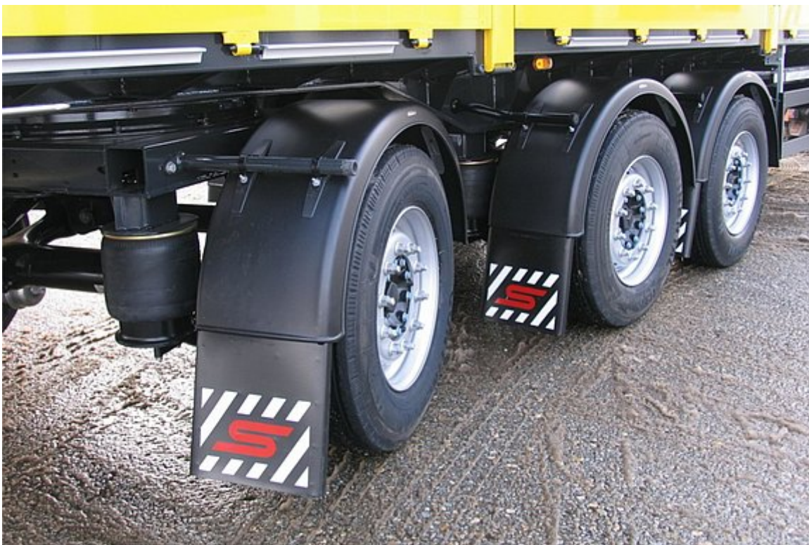
3. Semitrailer axle with mechanical forced steering
