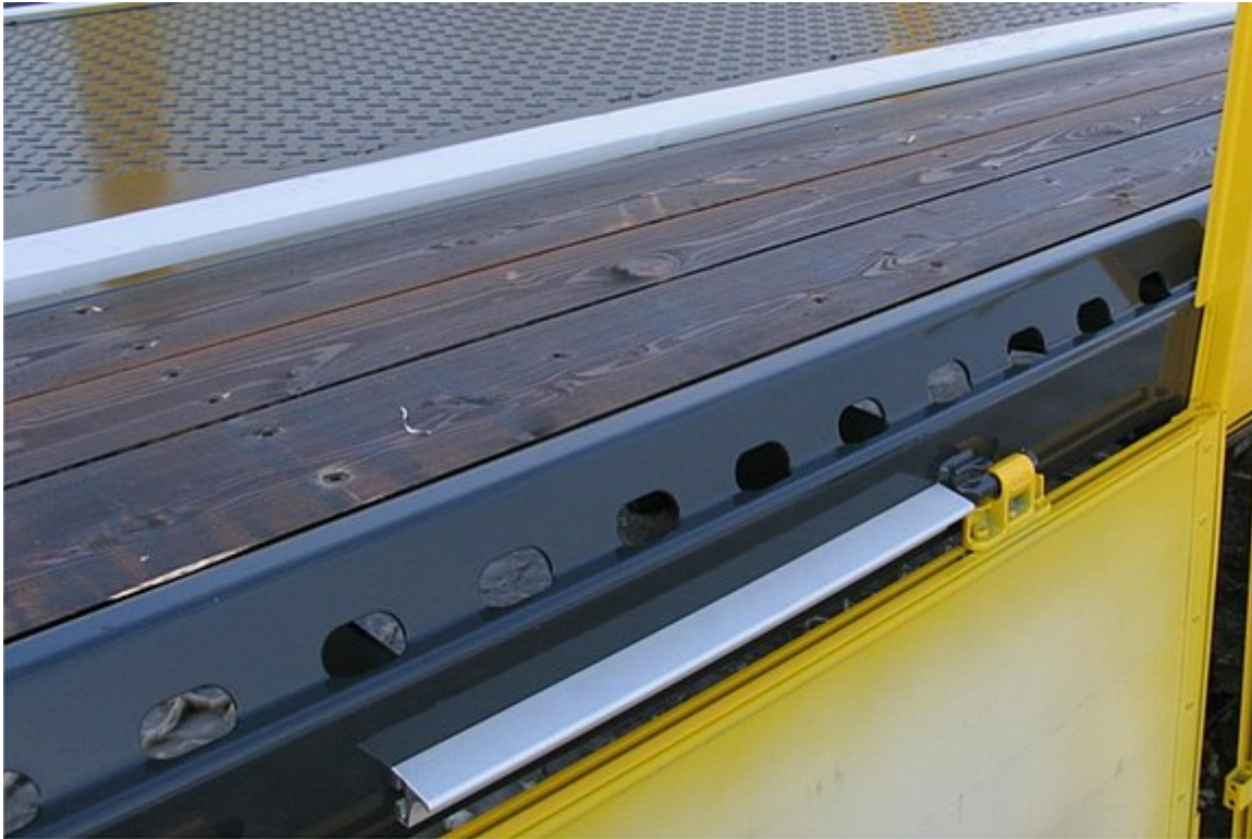
Perforated external frame with approx. 100 mm hole spacing, 50/30 mm slot, for securing 2 t
