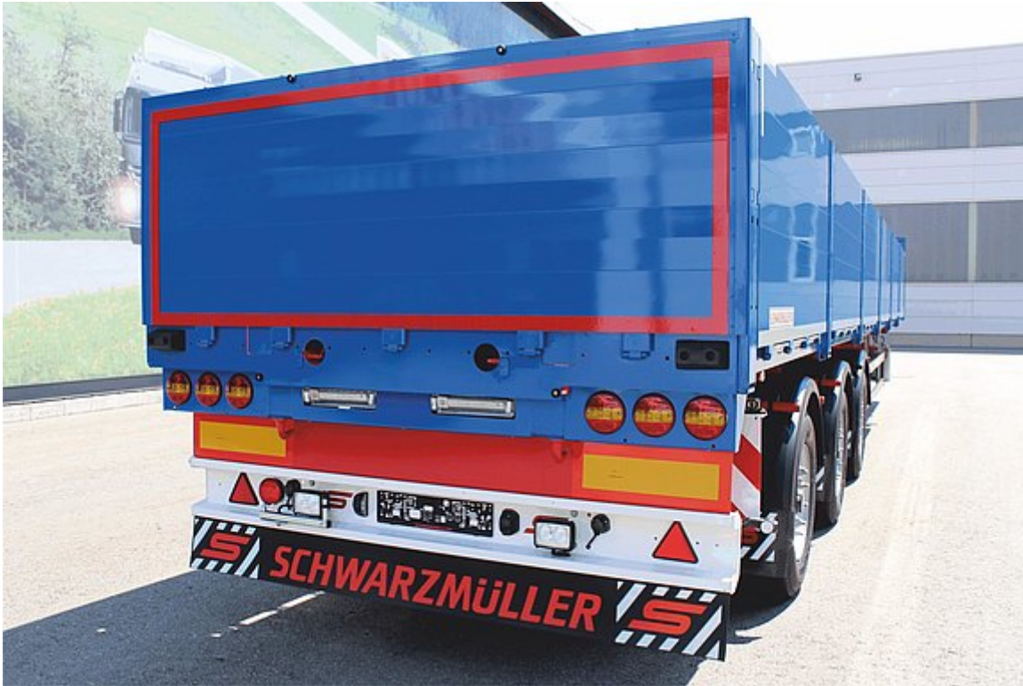
Reinforced, aluminium hollow profile rear wall, 1,000 mm high
