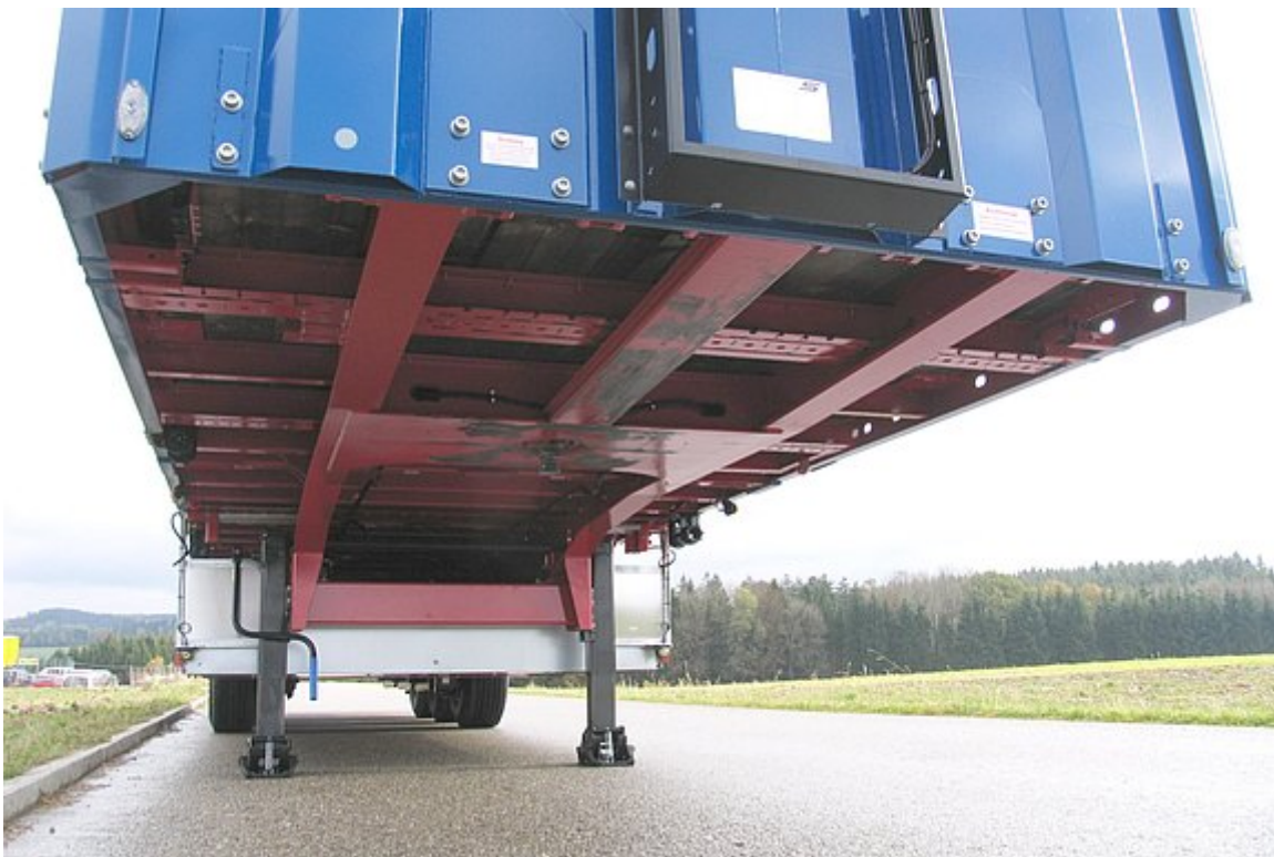
Torsionally rigid, welded ladder frame structure
