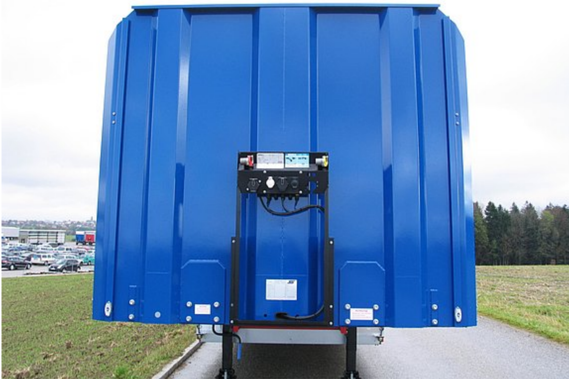
Profiled steel-sheet front wall
