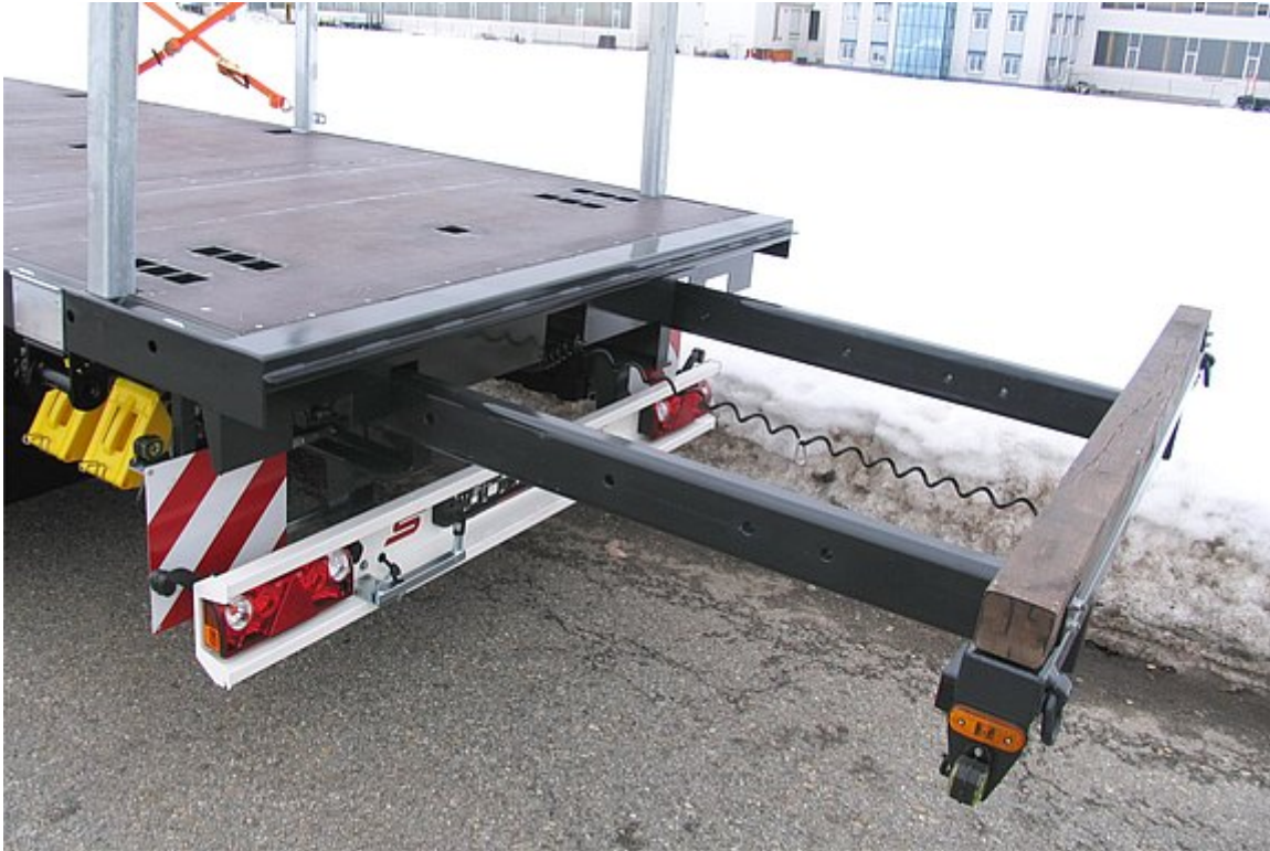
OPTIONAL: Rear pull-out frame, 1,500 mm (2 t load capacity)
