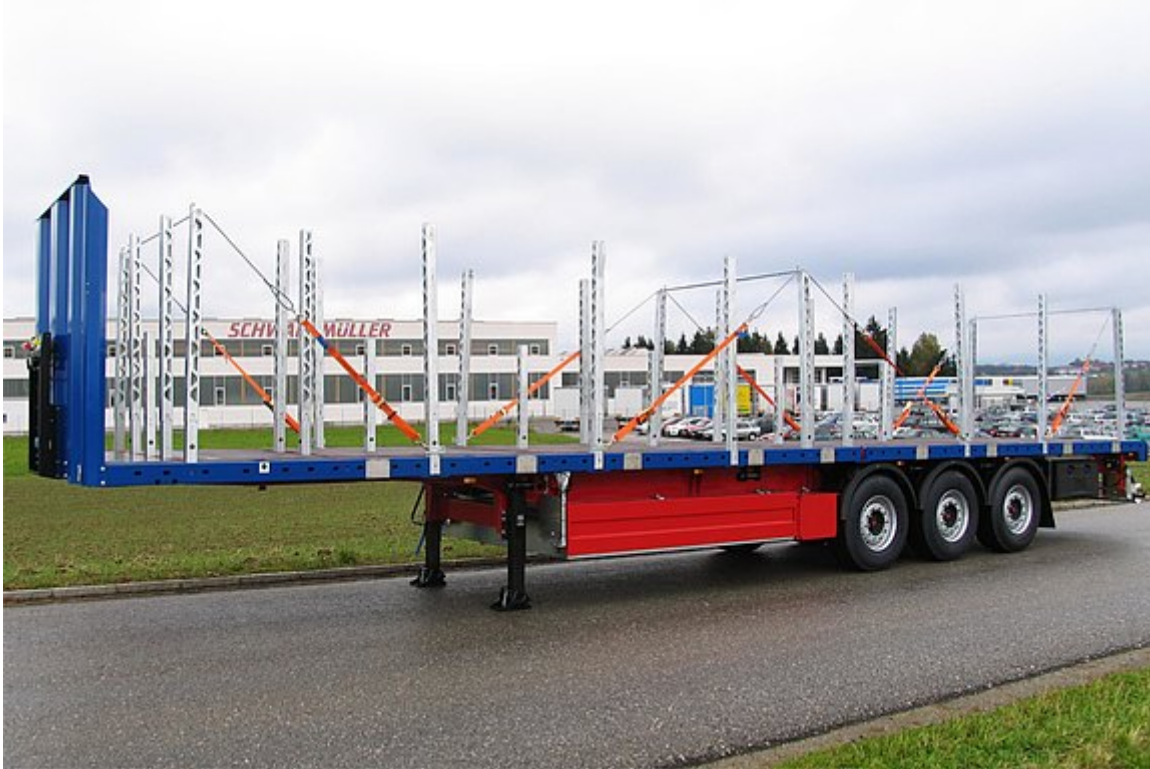
3-axle platform semitrailer for construction steel mat transport
