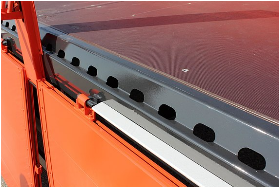
OPTIONAL: Perforated external frame with approx. 100 mm hole spacing, 50/30 mm slot, for securing 2 t per lashing point
