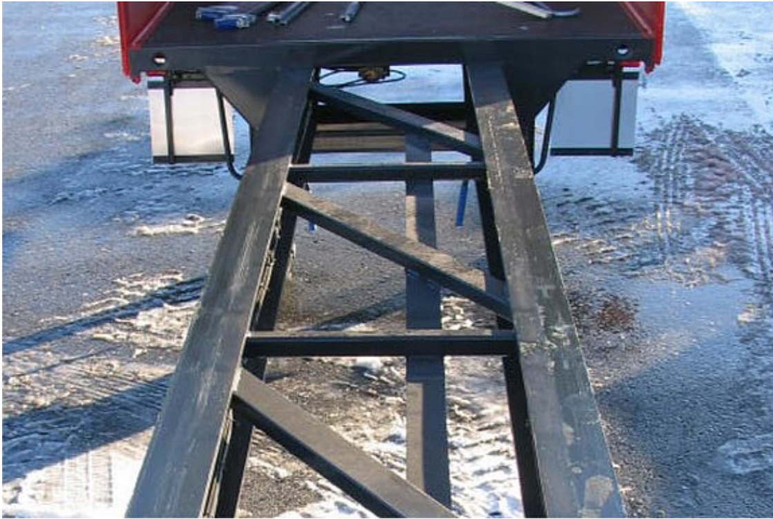
Extendible lightweight frame with an extension length of 6 m for long materials transport up to 22 m
