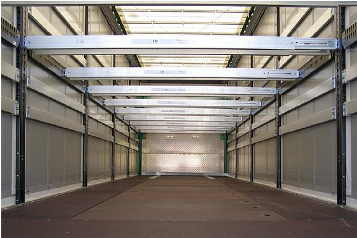
OPTIONAL: Twin-level loading system CTD III for 11 x 3 EURO pallets, load capacity: 400 kg/pallet
