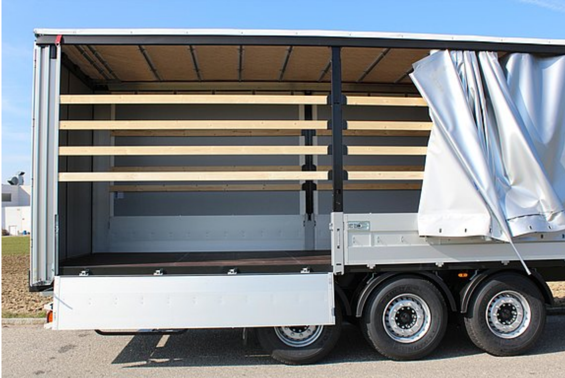
OPTIONAL: Version with sliding tarpaulin + side walls
