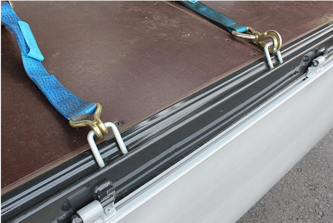
External frame with 15 pairs of recessed 2.5 t lashing points for load securing
