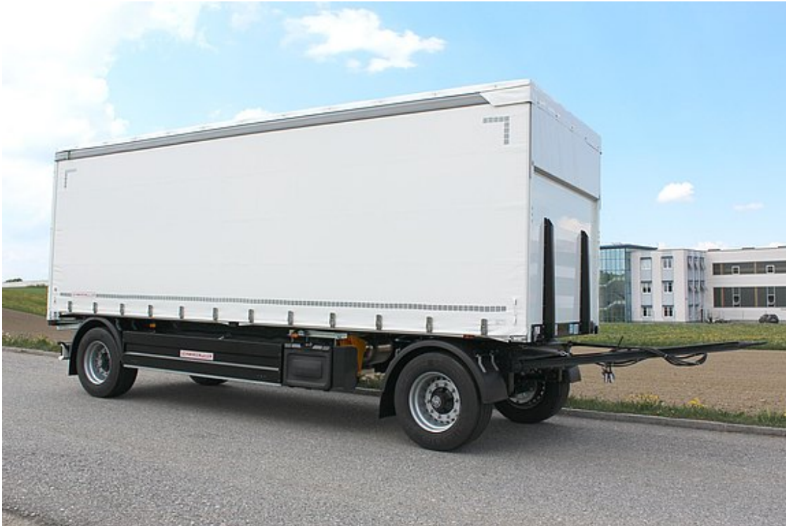
2-axle sliding tarpaulin platform trailer
