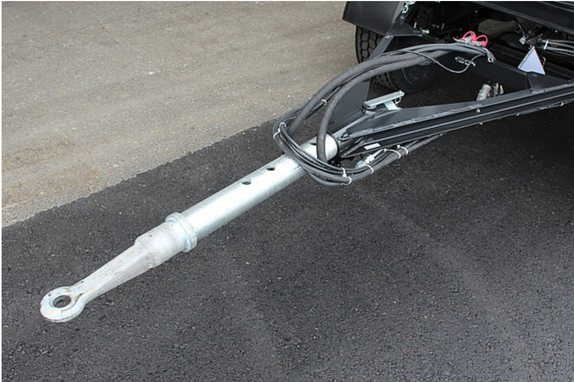
OPTIONAL: Pull-out drawbar, max. 600 mm adjustment, with Getofix drawbar support
