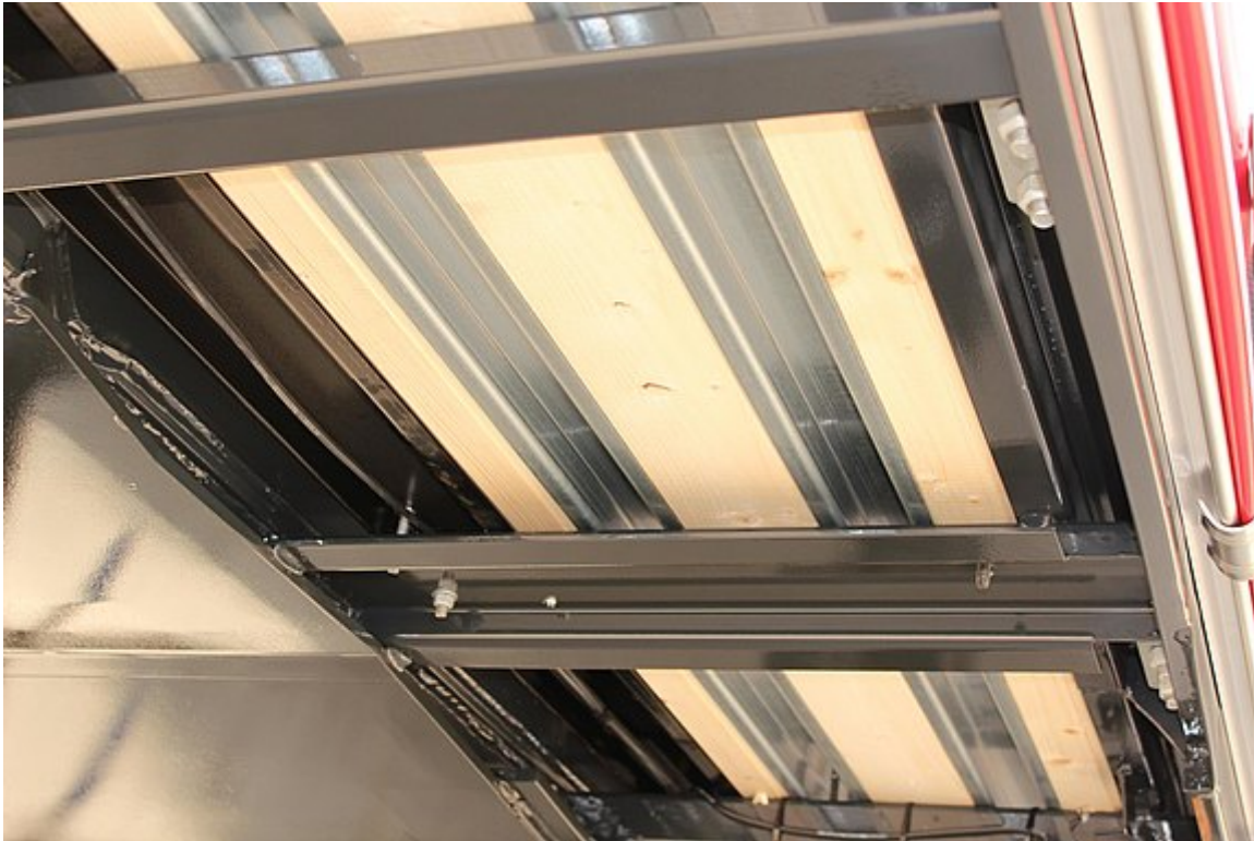
Double floor consisting of subfloor with integrated aluminium omega profiles beneath resin-coated wear floor or 27 mm resin-coated panel flooring behind
